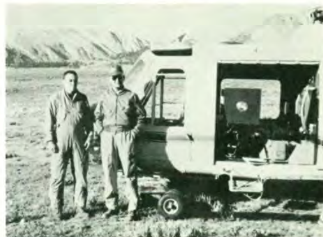
Test Pilot Dennis Tuck (left), and Flight Test Engineer Jim Thomason with the 204B at the Coyote Flats test site near Bishop, California. Note test instruments in cabin. Light is used to mark time of events with Fairchild camera.
