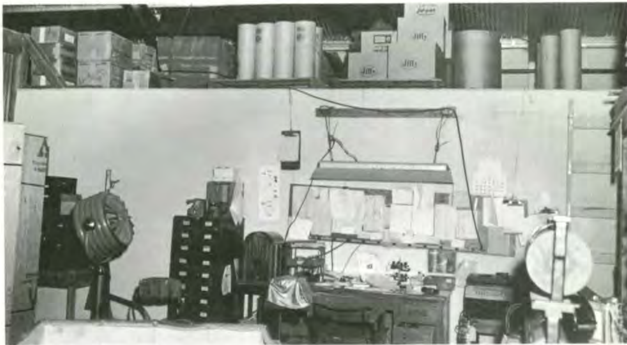
Can you spot the safety hazards in the above picture? Note improvised light fixture over desk, ladder at far right used for access to elevated storage area, and lack of guard rail around the storage area. Picture below shows the same area of the Warehouse after hazards have been eliminated. Ladder has been replaced by stairway with handrails, and guard rail and safe light fixture have been installed.
