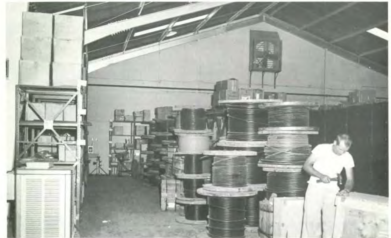
How safety improves efficiency: cable storage in top picture is unsafe, disorderly, and inconvenient. Below, steel racks installed for cable storage are safer, neater, handier, and permit three times as much cable to be stored in the same space.
