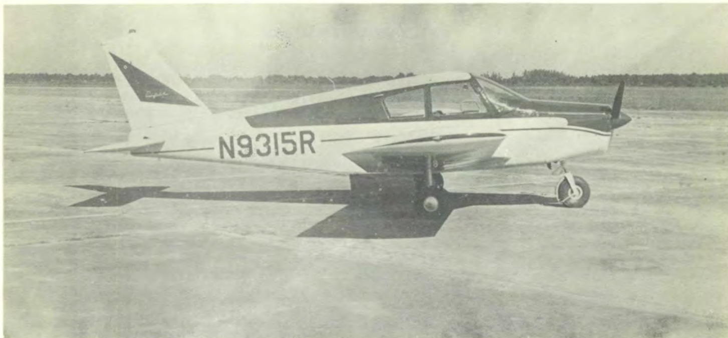
VERO BEACH, FLORIDA - Piper PA-28 "Cherokee" on ramp waiting further certification tests. Prototype has been flying since January 1960 at Piper Development Center.
