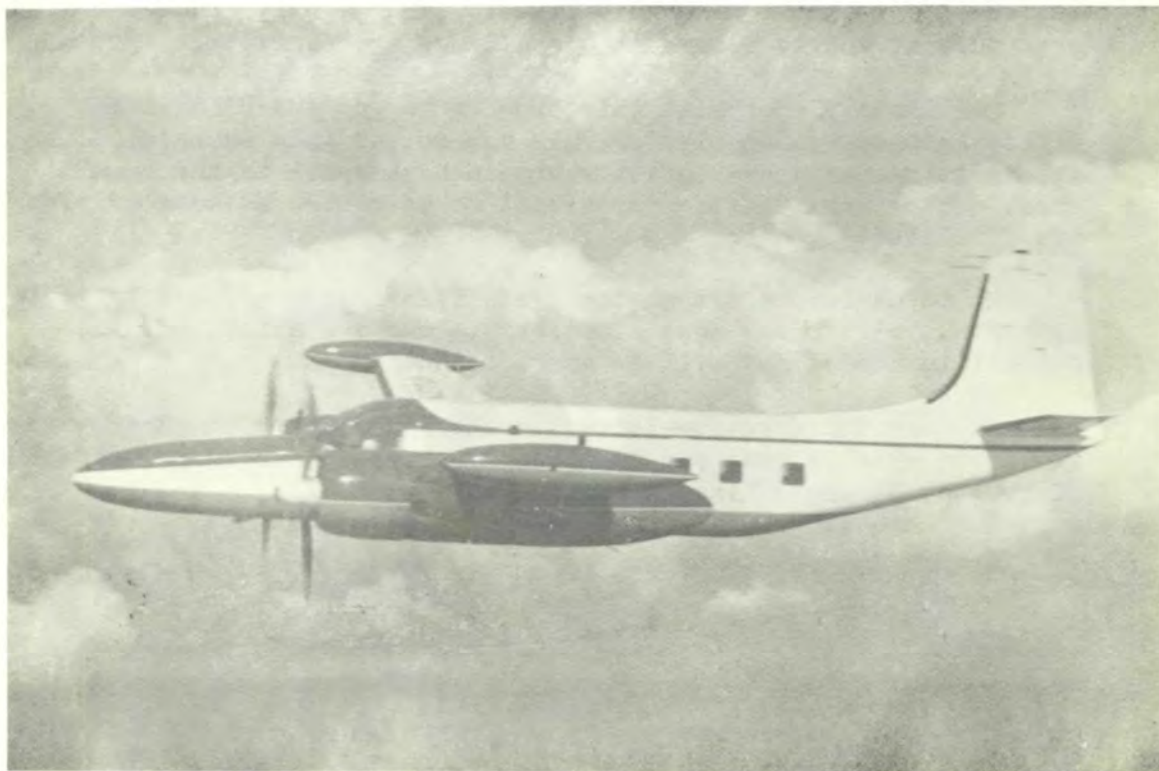
MIAMI, FLORIDA - L. B. Smith "Tempo II" in flight test by FAA engineering personnel. This aircraft was converted from a Douglas B-26 aircraft.
