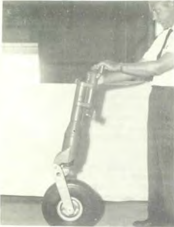
Nose gear is examined by D. E. Kemp, FAA Structures Engineer, prior to gear drop tests.
