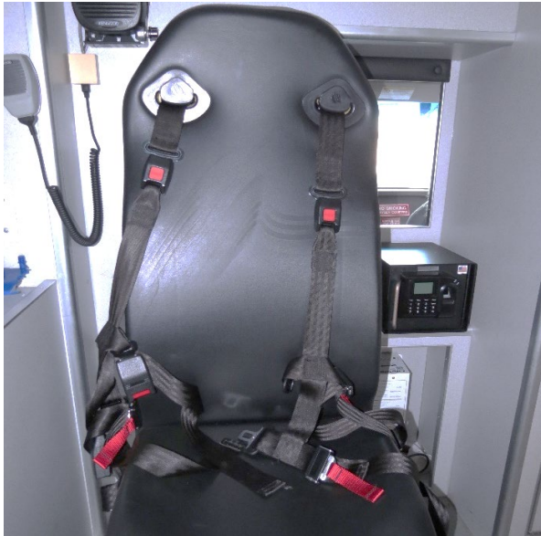
Figure 16. Viewing the belt systems of the captain's chair
