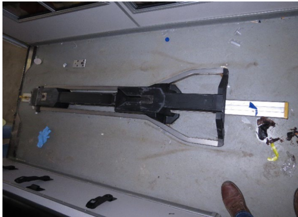
Figure 19. View of the cot latching system
