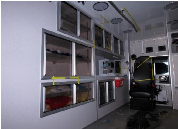
Figure 12. View of the left rear of the patient's compartment (tape at the left bottom indicated the soft tissue contacts to the aluminum trim)
