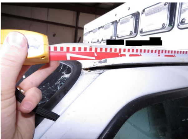
Figure 8. Left side roof weld fracture
