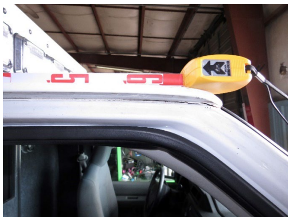
Figure 9. Right side roof weld fracture
