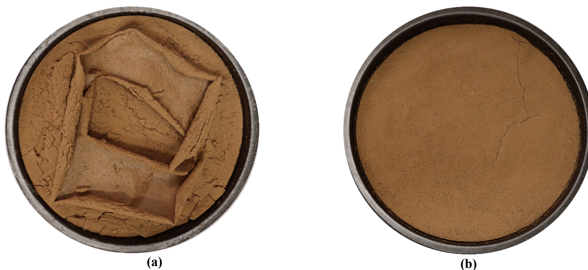
Figure 2-5. Appearance of dried treated surface by a) regenerated normal starch hydrogel (RNSH), b) regenerated amylopectin starch hydrogel (RASH)
