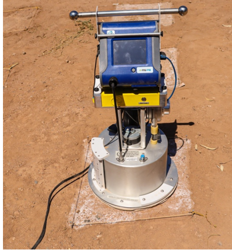
Figure 3-1. Portable in-situ Wind Erosion Lab (PI-SWERL) test device.
