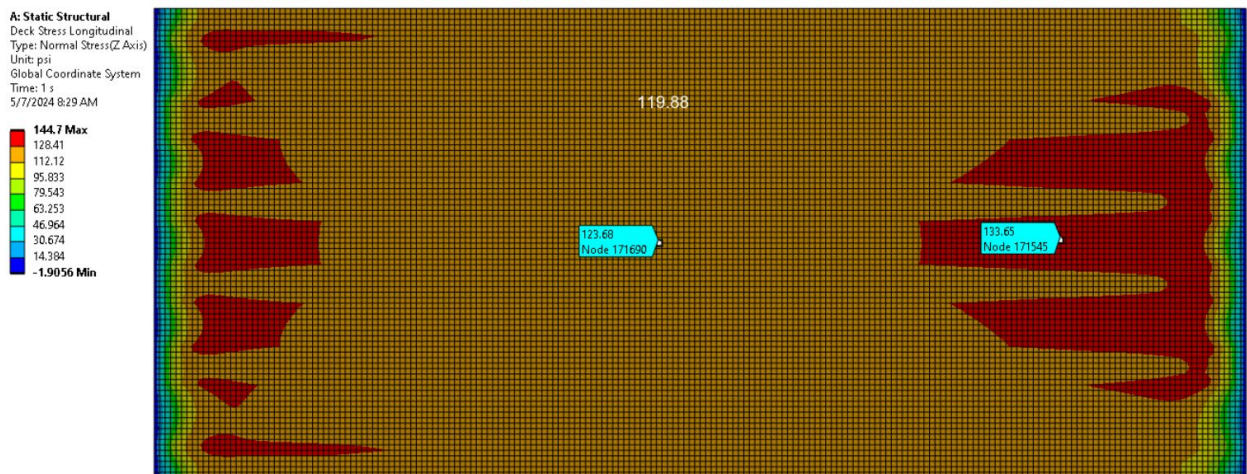
Figure 5.1.3. Bridge deck longitudinal stresses due to negative thermal gradient
