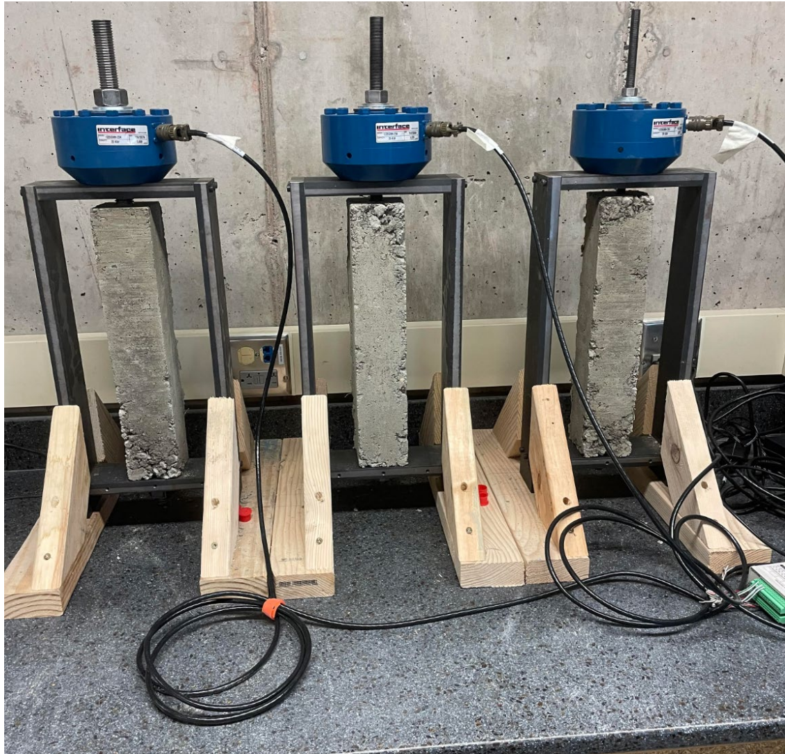
Figure 3.2.3. Restrained shrinkage tests in operation
