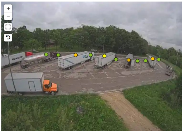
Figure 2. Camera picture of the Heath Creek truck parking area. Occupied parking has a green dot and unoccupied has a yellow dot. The dots are a computer count on available open spots to communicate by the 511 map.
