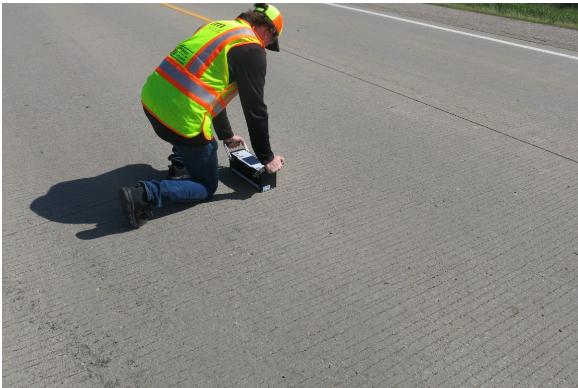
Figure 5.7 Pavement subsurface condition evaluation using ultrasonic tomography.
