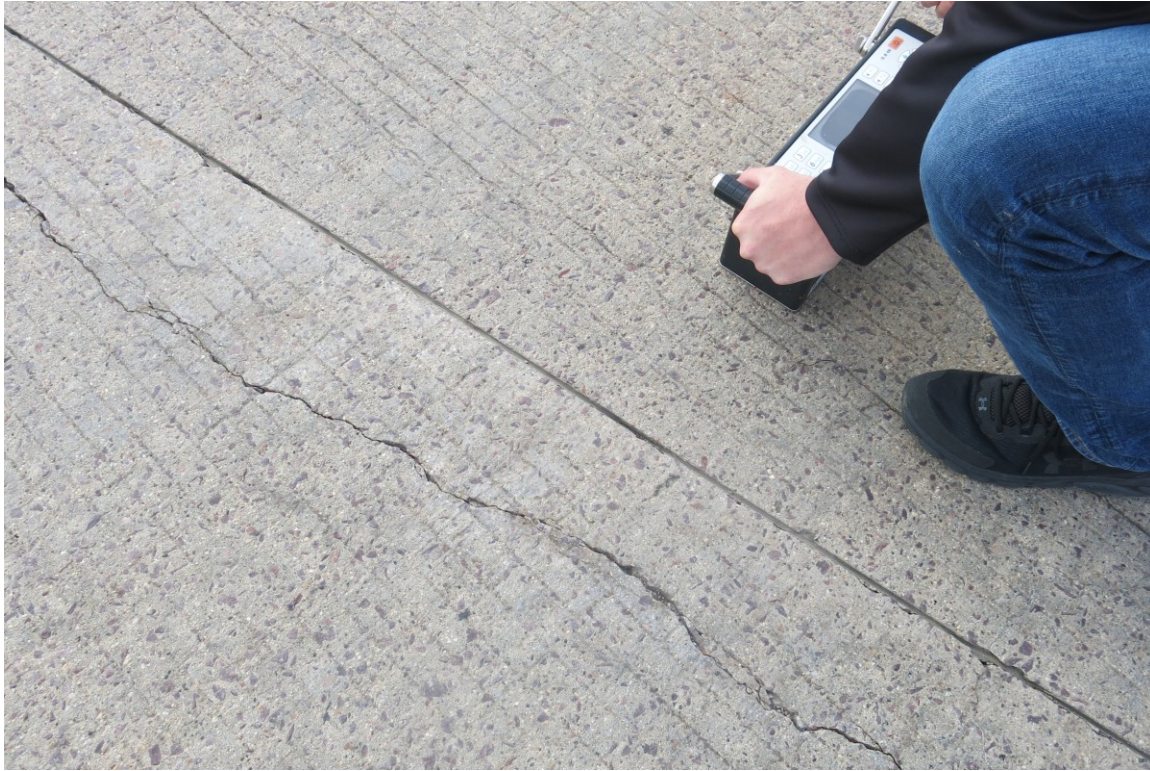
Figure 5.6 Pavement subsurface condition evaluation using ultrasonic tomography.
