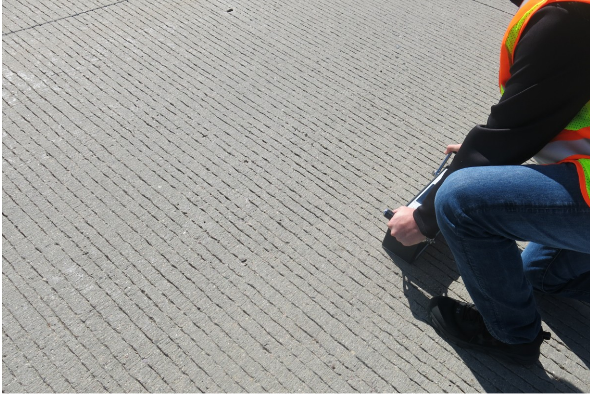
Figure 5.8 Pavement subsurface condition evaluation using ultrasonic tomography.
