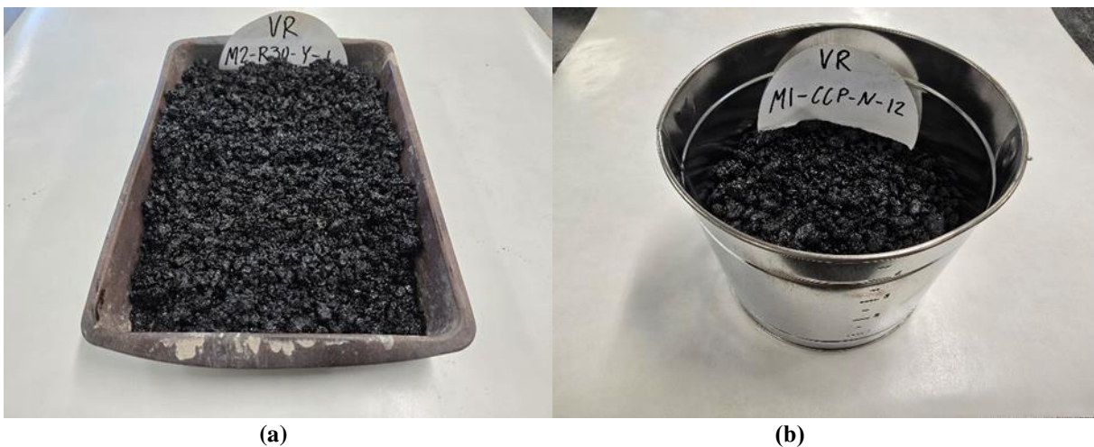
Figure 8. Container Types Used for Evaluating Loose Mixture Specimen Thickness in Containers: (a) Shallow Pan; (b) 5-Quart Pail
