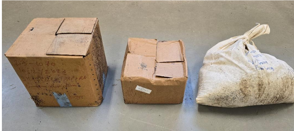
Figure 12. Containers Evaluated for Heating Time Effects (left to right): Virginia Transportation Research Council's 10 × 10 × 10-Inch Box, 10 × 10 × 6-Inch Box, and Canvas Bags Used in VDOT Field Sampling.
