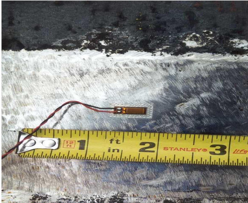
Figure 2. Pile gages were weldable quarter-bridge Micro Measurements strain gages supplied by Vishay Instruments. Gages are 7/16 in long and attached by micro-spot welding a 5/8 in long thin steel backing to a ground and cleaned steel surface. These micro-spot-welded gages are more reliable in translating strain from the steel substrate than with gages using bonding adhesives, which frequently debond during loading, or have limited fatigue life after sustaining frequent large strains during service.
