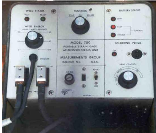
Figure 3. Strain gages were attached by micro-spot welding the thin steel sheet backing of the resistance wire using a Micro Measurements Model 700 portable strain gage welding and soldering unit. Weld input energy in joules is varied to control the depth of spot weld penetration, similar to methods used in conventional resistance spot welding of metals.
