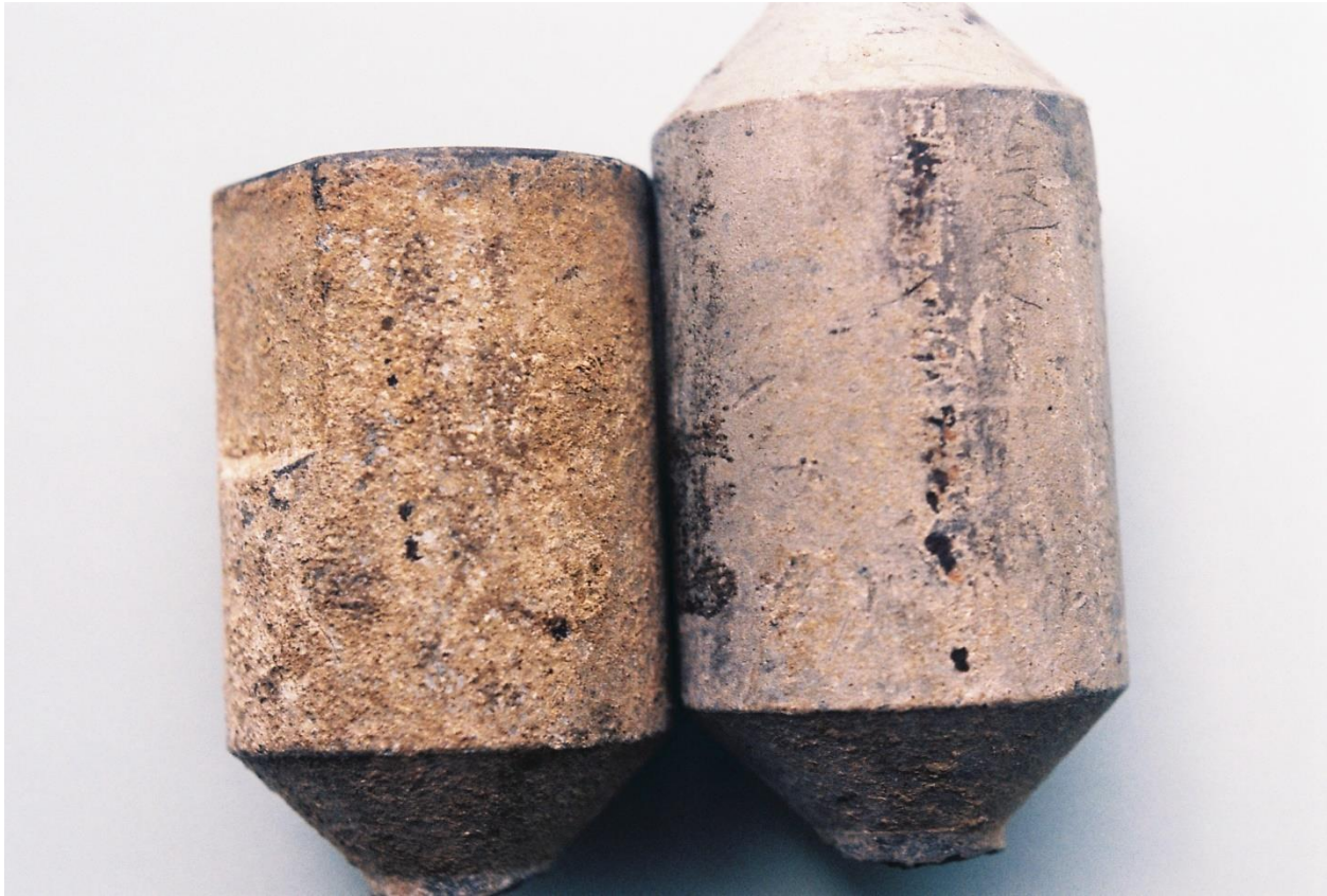
Figure 7. The zinc coatings on the couplings had degraded by forming zinc oxides and chlorides (oxides are white and yellow; chlorides are white) as a function of long-term exposure to moisture, salt spray and the accumulation of dirt and debris. Note the formation of pits in the sides of the couplings when the zinc coating was depleted. Pits also formed at notches, leading eventually to deeper cracks.
