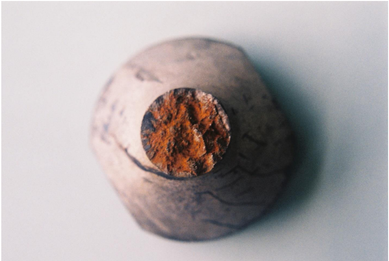
Figure 15. The third coupling has incipient initial fatigue cracks at the 8:00 to 10:30 clock position but exhibits relatively faster crack propagation fracture surfaces as loads were
