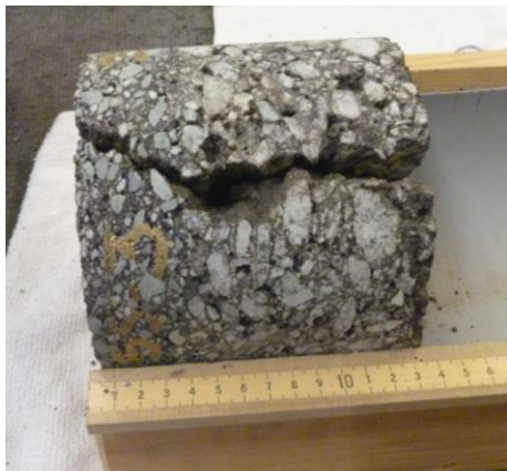
Figure 12. Section K, SR 631N, Core 4 Showing Bottom-up Fatigue Cracking.
