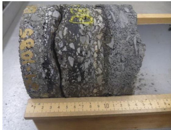
Figure 10. Section B, SR 685S, Core 21 Showing Delamination.
