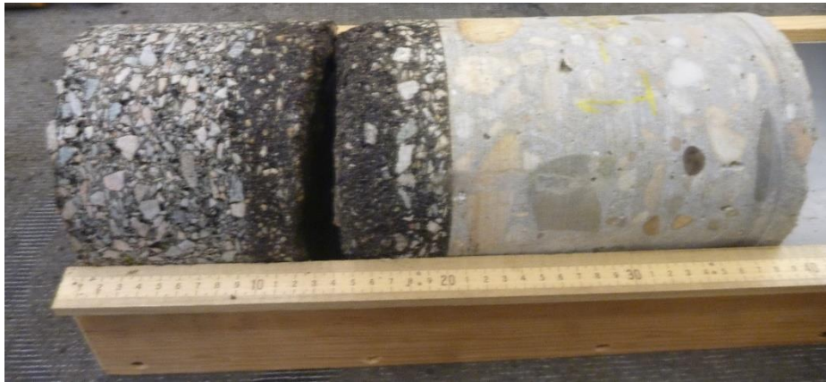
Figure 11. Section G, US 1S, Composite Pavement Core 1 Showing Stripping and Delamination. Most cores were extracted with the bottom surface in the dark delaminated layer, likely indicating that the layer has a stripping issue.
