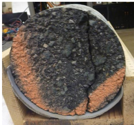
Figure 13. Section K, SR 631N, Core 5 Showing Top-down Cracking
