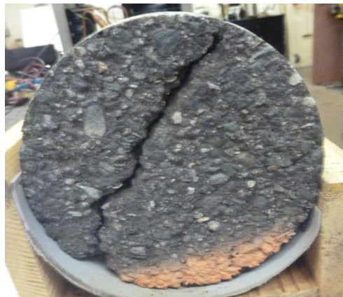
Figure 12. Section K, SR 631N, Core 4 Showing Bottom-up Fatigue Cracking.
