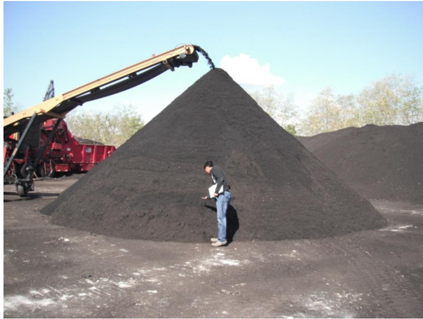
Figure 3: Stockpiling Finely Ground 0.25-inch RAS Particles. [Source: IDOT Photo – Waste Commission of Scott County, Davenport, Iowa]
