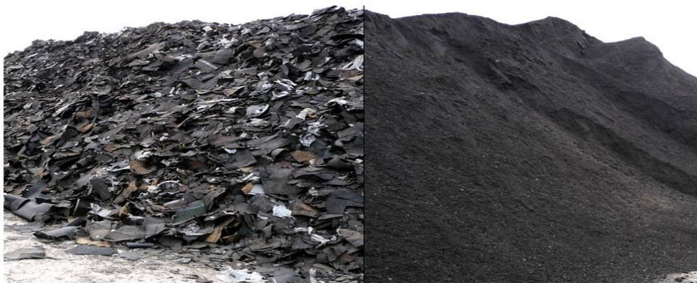
Figure 2: Raw Post-Consumer Shingles (Left) and Processed RAS (Right). [Source: http://www.roofingshinglerecycling.com/ ]
