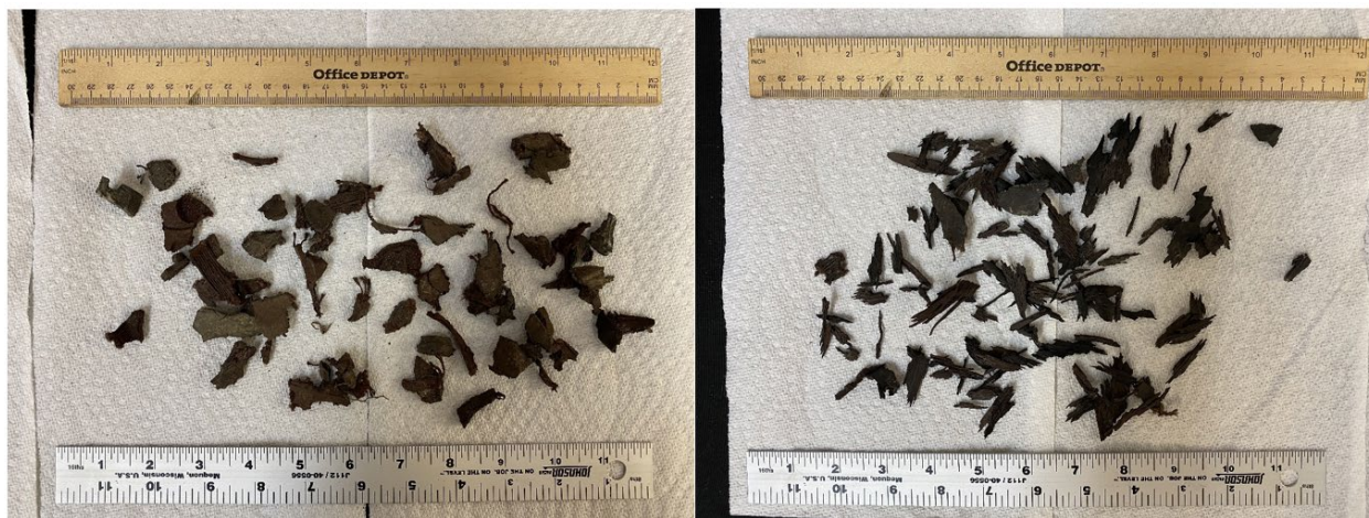
Figure 16. Pictures of two TDA materials used for PFAS leaching test. On the left are the wire-off TDA rubber nuggets, and on the right are the wire-off shredded TDA rubber.
