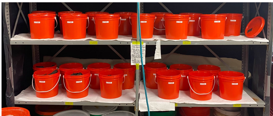
Figure 2. Experimental setup of batch buckets with TDA kept at room temperature at SAFL. Top shelf: batch buckets with Lid-on treatment, bottom shelf: batch buckets with Lid-off treatment.
