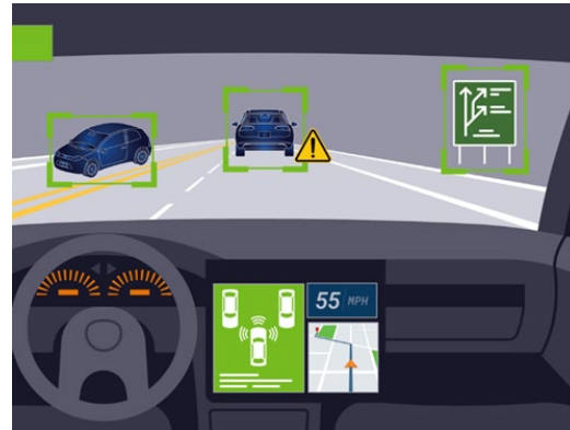
Figure 1. Illustration of machine vision detecting roadside assets, such as traffic signs.
