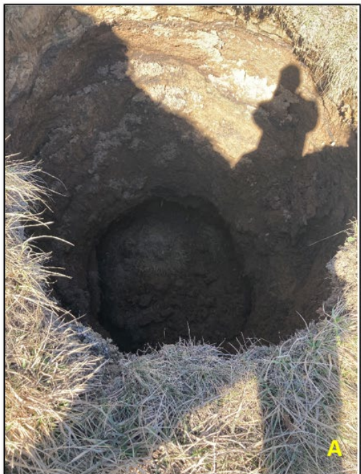
Figure 4: a- Suspected mine shaft opening on US 63 south bound near shoulder, March 2021.
