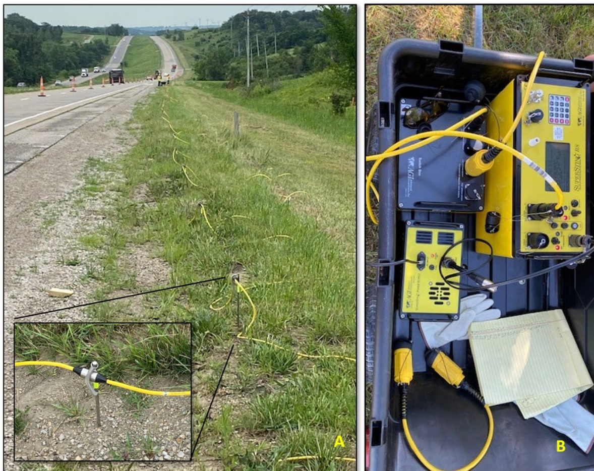
Figure 7: A. View of ER survey line showing location near US 63 and electrode spacing of 13 feet between each electrode. A close-up view of a single electrode is shown in the lower left corner. B. AGI Super Sting unit, the set up was transported in a field cart.
