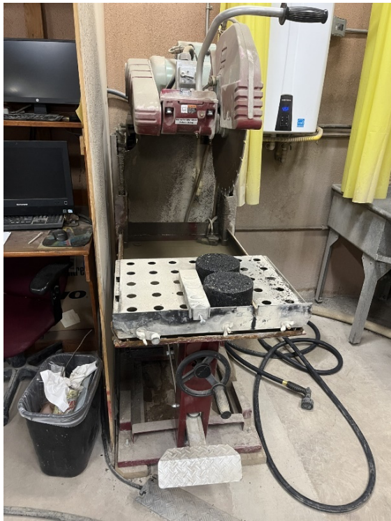
Figure 2.11. Saw-Cutting Specimen Along its Edge
