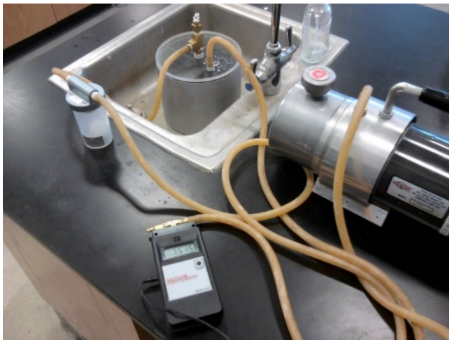
Figure 2.6. Vacuum Saturating a Loose HMA Specimen for TMSG
