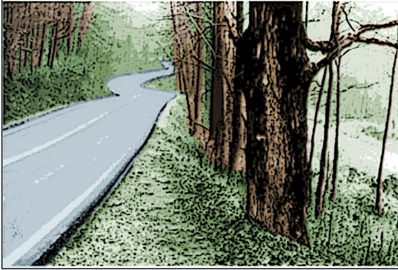
Figure 32. Graphic. Illustration of a Roadside Rating 6.
