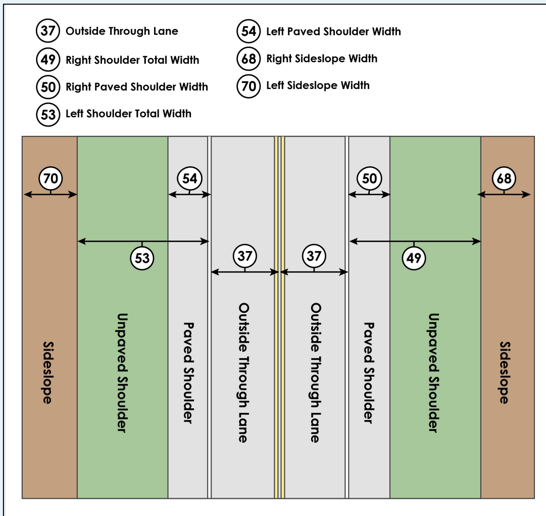
Figure 15. Graphic. Illustration of cross section, two-lane roadway.
