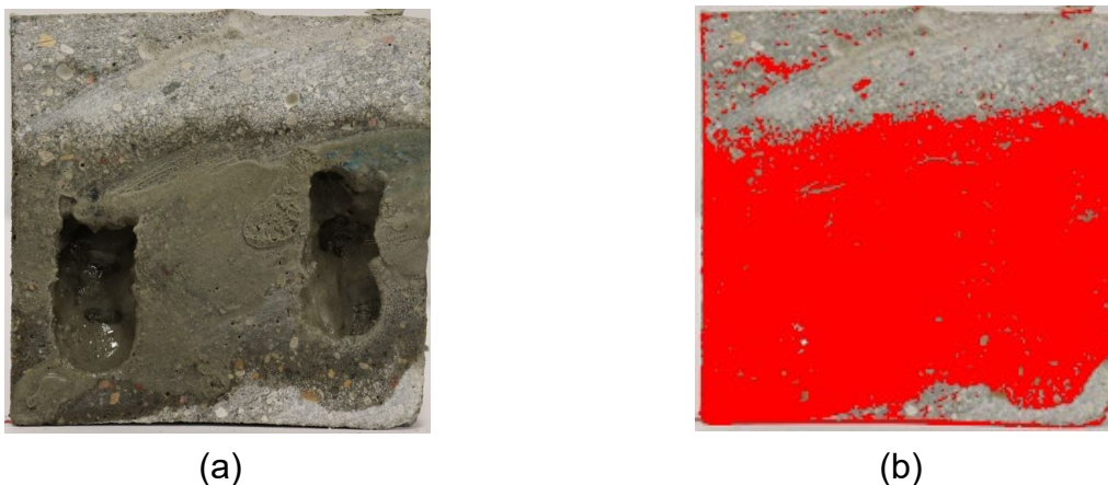
Figure 2.4: (a) Picture of a sectioned mortar cube after 1-day of curing with 1%-HB capsule under gravity force, and (b) wet area color coded as red by the ImageJ software.
