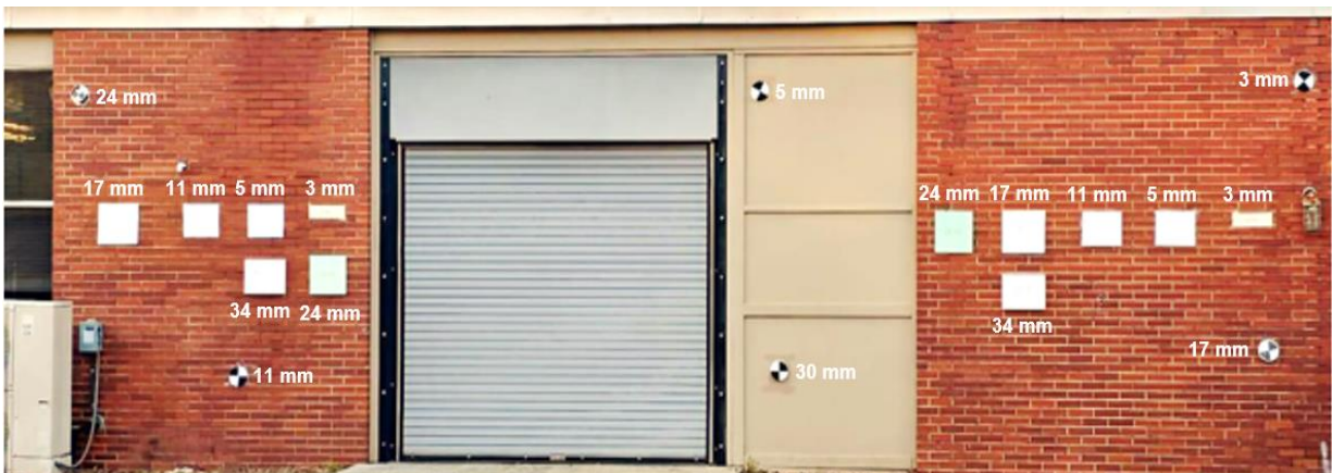
Figure 40. Photo. Styrofoam Inserts Simulating Displacements at CW
