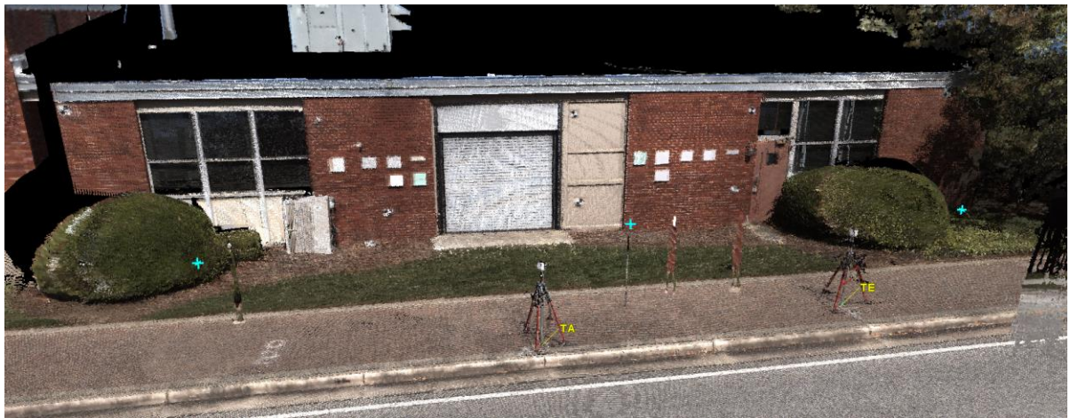
Figure 28. Photo. TB LiDAR point-cloud model of deformed CW in Epoch 2
