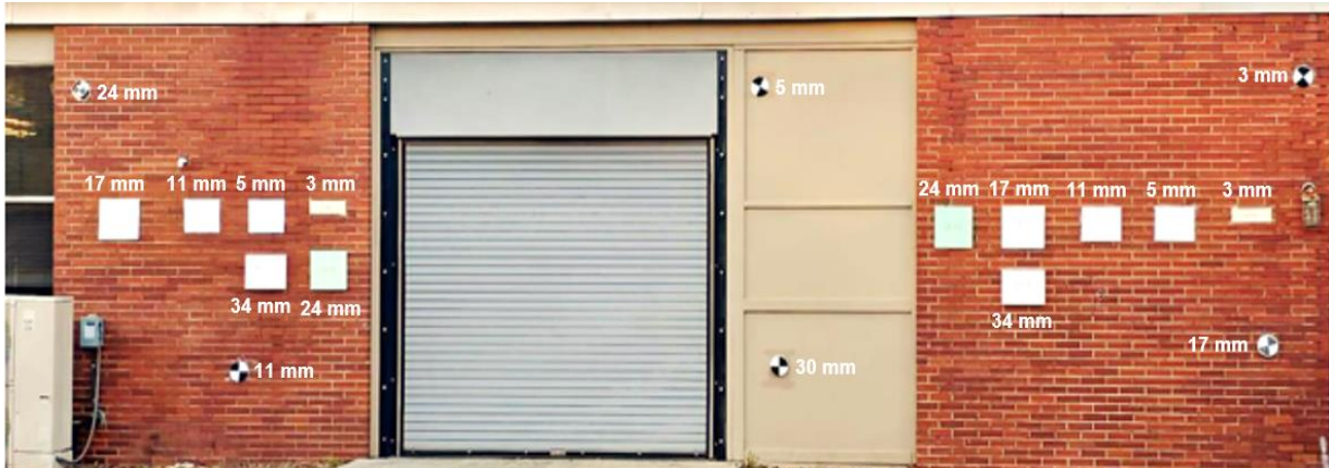
A. CW with simulated displacements and their magnitudes at Epoch 2.
