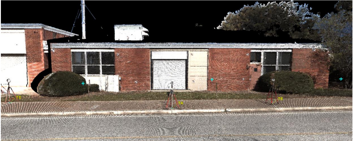
Figure 27. Photo. TB LiDAR point-cloud model of the undeformed CW in Epoch 1
