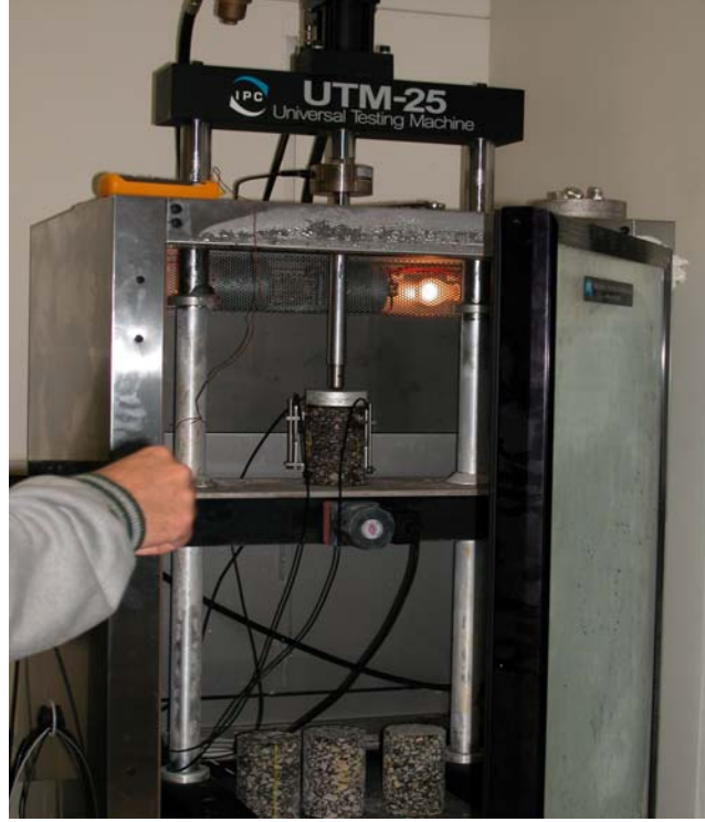
Figure 4.1. Dynamic Modulus Testing Setup.
