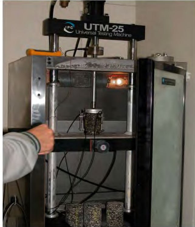
Figure 2.3. UTM Machine Used for Simple Performance Tests.
