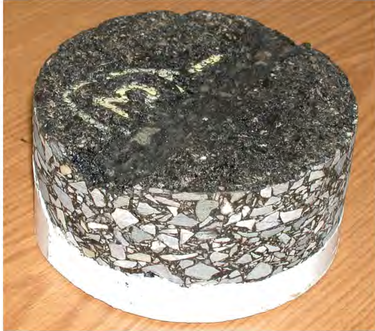
Figure 8. Modified Roadway Core Specimen after APA Testing.
