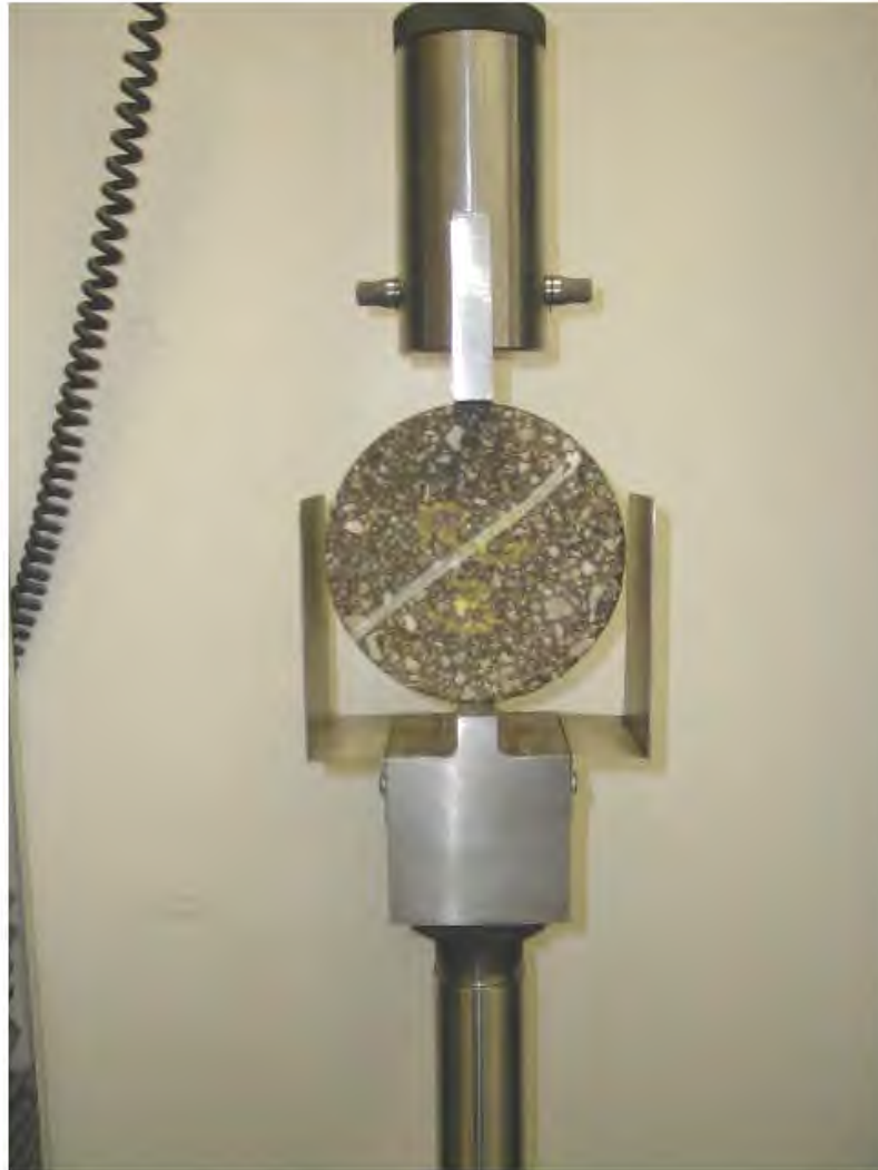
Figure 9. Indirect Tensile Strength Test Setup.
