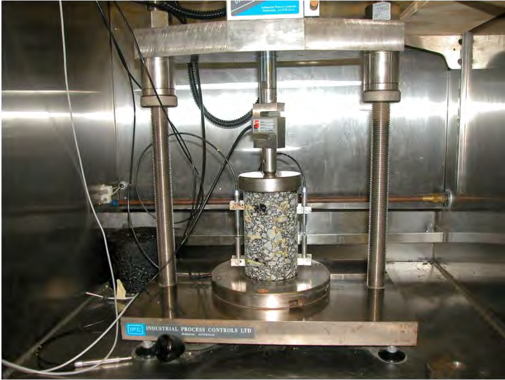
Figure 10. Dynamic Modulus Testing Setup.
