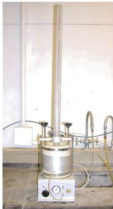
Figure 5. Florida Permeability Test Setup.
