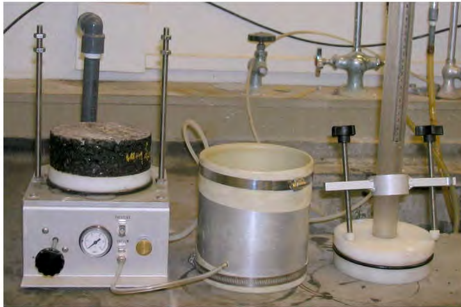
Figure 4. Florida Permeability Test Apparatus.
