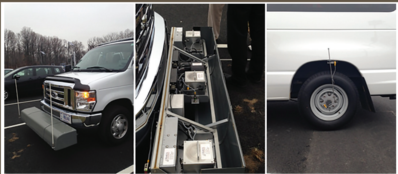
Figure 9. Inertial profilometer vehicle (left), sensor bar with cover open (center), and distance measurement instrument (right).
