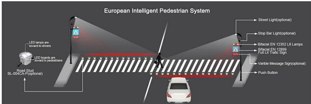
Figure 5-9. European Intelligent Pedestrian System. Source: Ellumin
