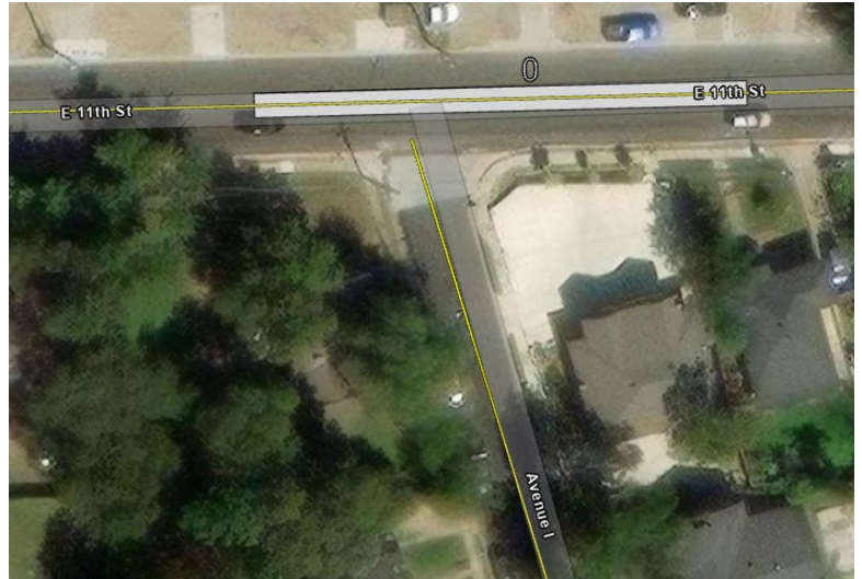
Figure 6-3. 50-meter piece incorrectly classified as not having a tee ('tee_or_int' label shown as 0), due to polylines not connecting at intersection. The branch of the tee does not fall inside the white rectangular buffer
