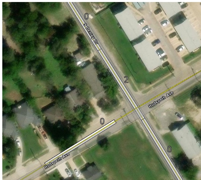
Figure 6-2. The value of 'tee_or_int' shown for a few 50-meter records, shown as thin white rectangular 1.25-meter buffers. Roadway polylines are yellow
