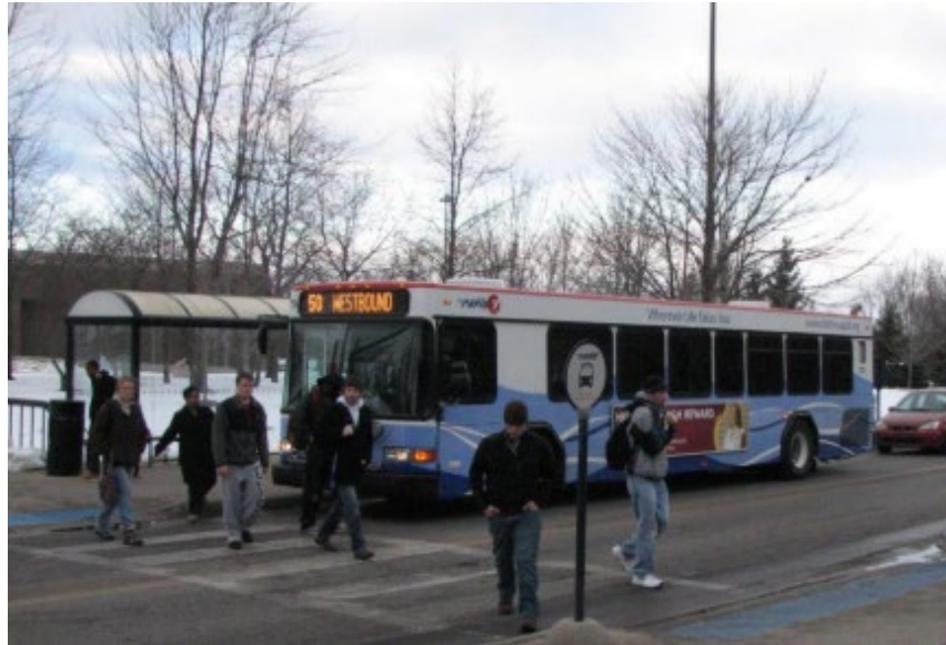
Figure 2-15. Bus obscuring vision of pedestrians in crosswalk (Image: Cox, N., and Prudhomme, C. 2014)
