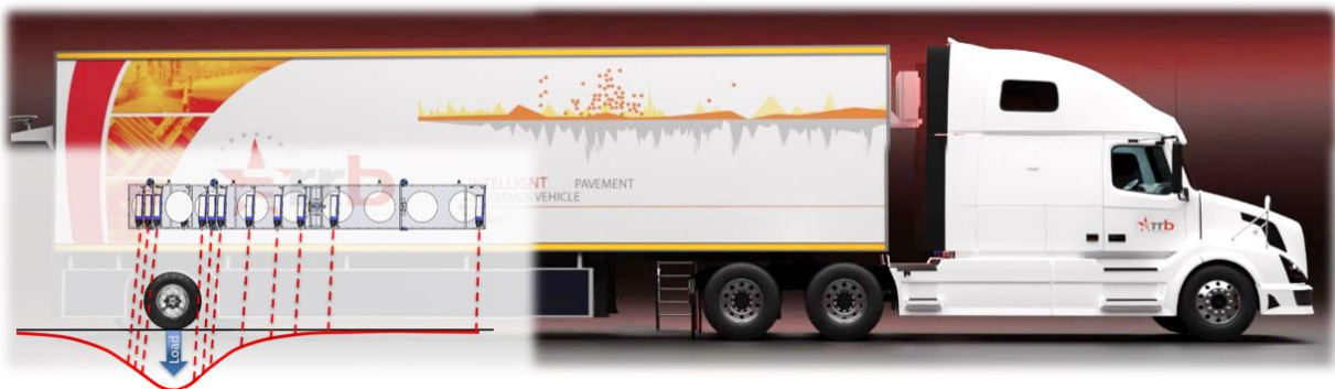
Figure 1. Traffic Speed Deflectometer with Doppler Lasers Mounted on Measuring Beam (Provided by ARRB Systems USA, used with permission)
