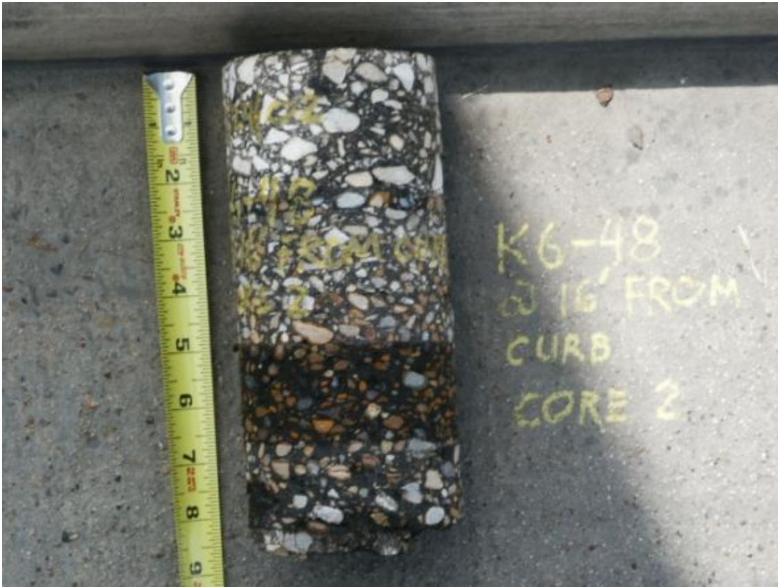
Figure 6.22. Intact Core Taken from Vicinity of K6-48.
