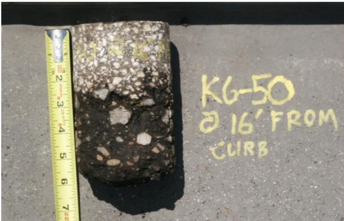
Figure 6.21. Piece of Broken Core Taken from Vicinity of K6-50.
