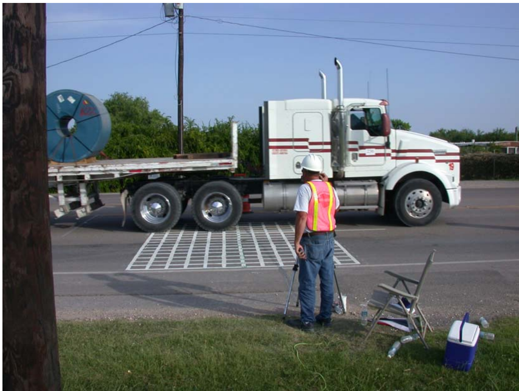
Figure B20. Permitted Truck Going Over MDD on K7 Lane.
