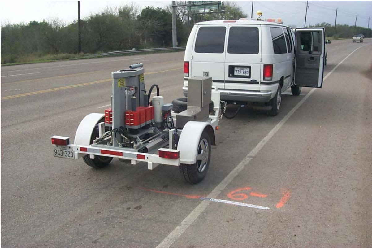
Figure 2.3. Falling Weight Deflectometer.
