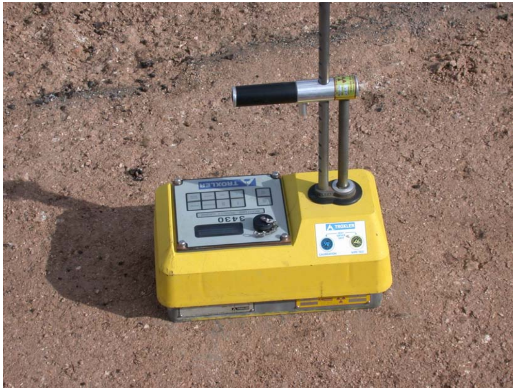
Figure B4. Density Measurement on Base Material.
