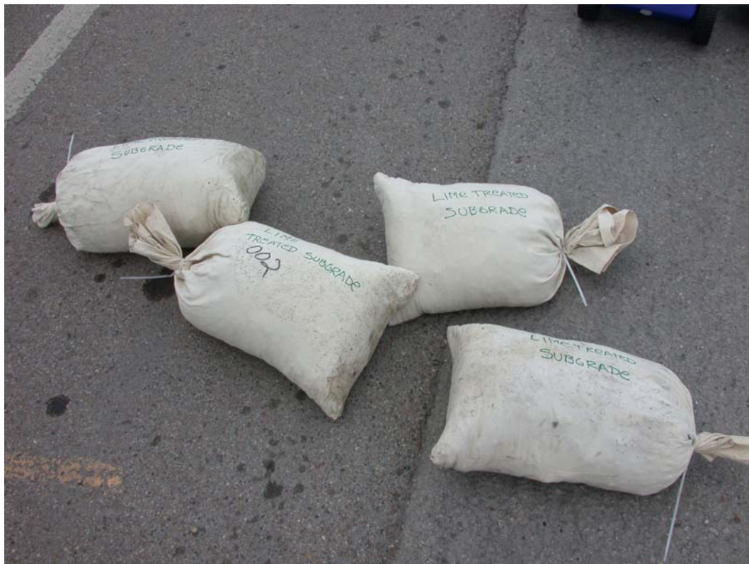
Figure B5. Samples of Lime-Treated Subgrade Collected from WIM Site.
