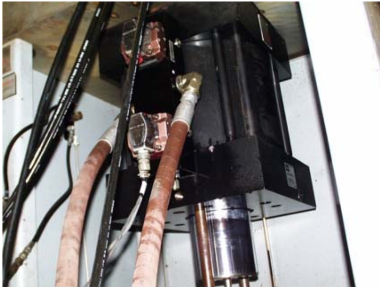
Figure 3-3: MTS Hydraulic Actuator
