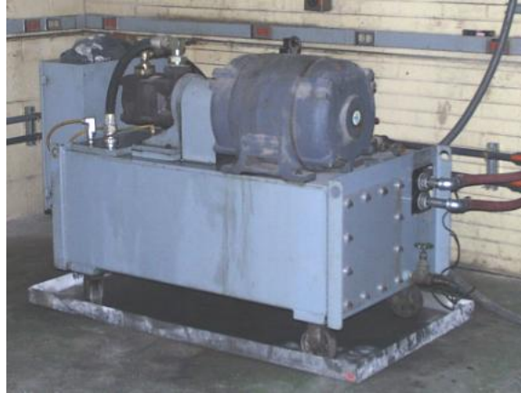
Figure 3-4: MTS Hydraulic Supply Unit
