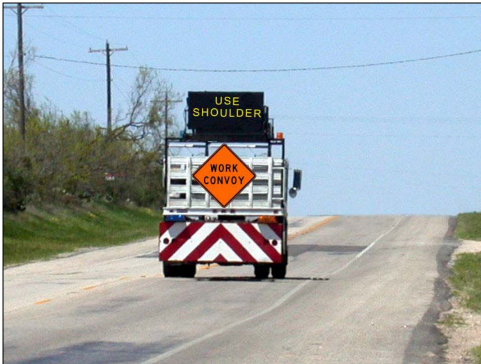
Figure 26. Use of a USE SHOULDER CMS Message.
