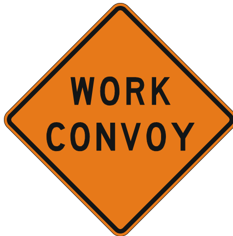
Figure 3. WORK CONVOY Sign (CW21-10).
