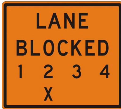
Figure 10. LANE BLOCKED Sign (FCW20-6).
