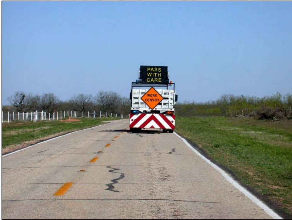
Figure 19. Use of a PASS WITH CARE CMS Message.
