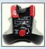
Additionally, the incoming oxygen is diluted with cabin air and provides the proper percentage of oxygen, depending on the altitude. This system is typically used at altitudes up to 40,000 feet.
