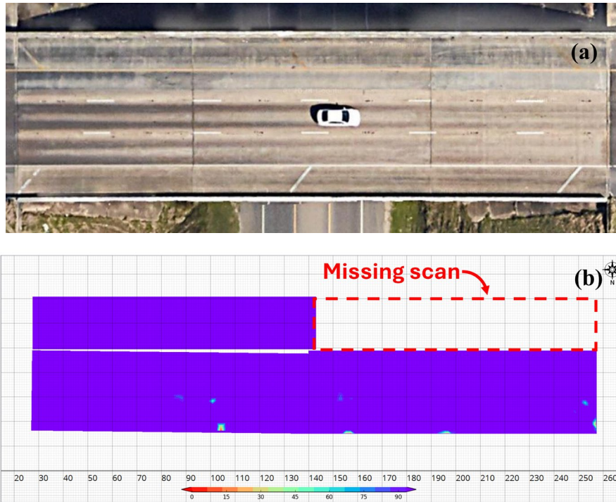
Figure 8.3 Example of NDE condition map with missing scans: (a) actual bridge image from Google Maps; (b) ER map from LTBP showing missing scan areas caused by automated scan self-termination (LTBP).
