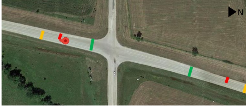
Figure 3.2: Approximate Superelevated Transitions at 169-2 RP 79.2
