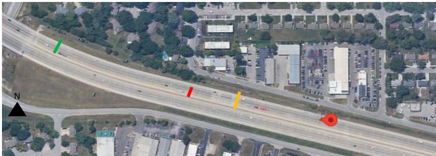
Figure 3.5: Approximate Superelevated Transitions at 35-46 RP 217.55
