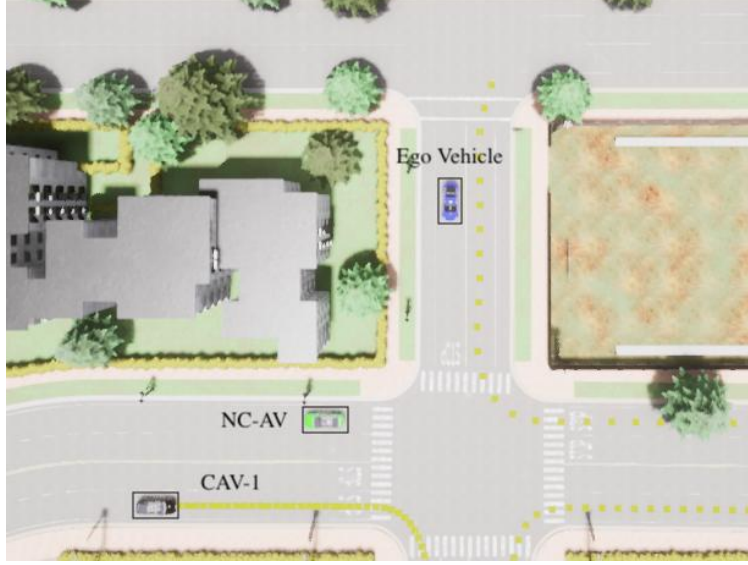
Figure 3.5: Intersection Scenario with Lane Change Based Obstacle Avoidance
