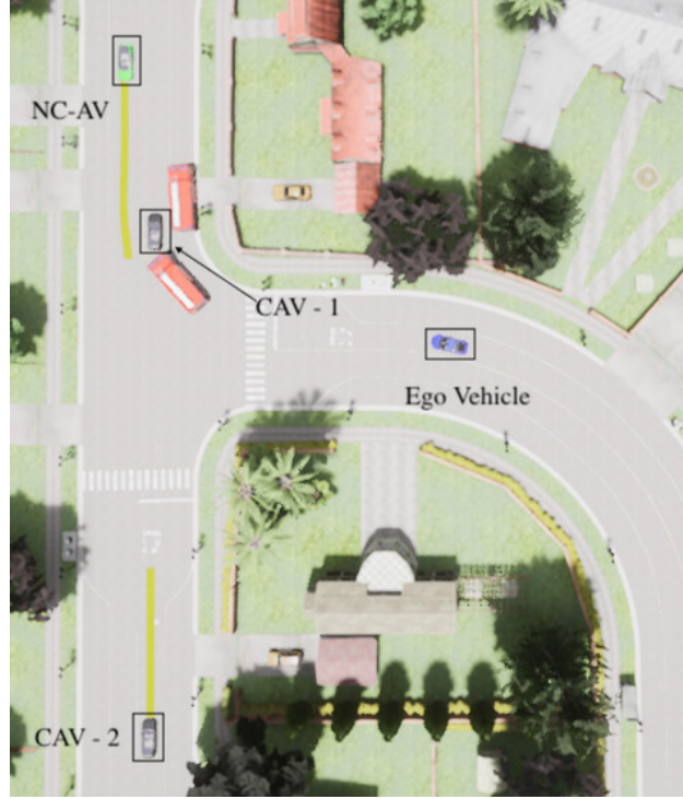
Figure 3.4: Cooperative Perception at a T-junction: Connected vehicles CAV-1 and CAV-2 share their observations of the non-connected vehicle NC-AV with the ego vehicle.
