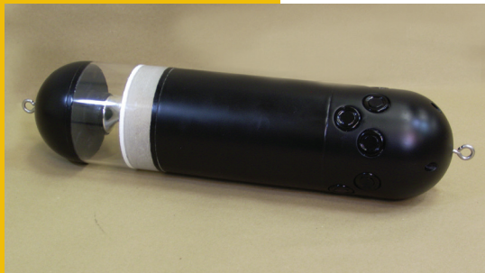
The prototype culvert inspection probe.
