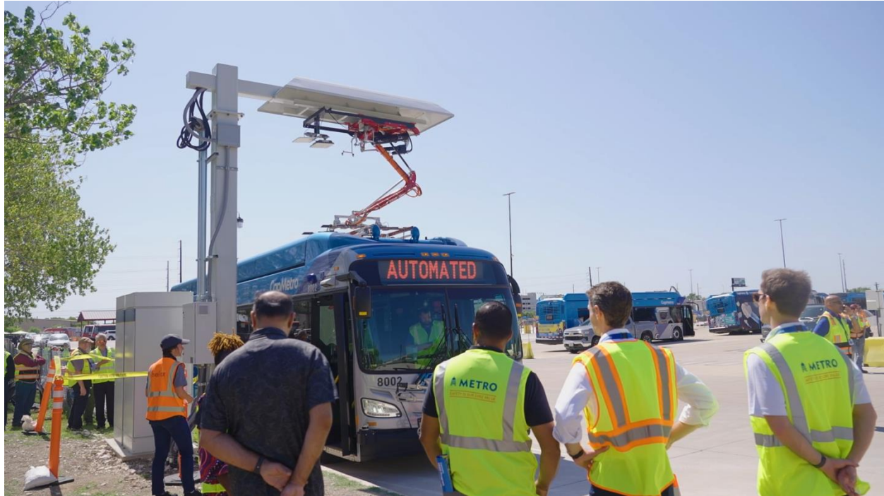
Figure 1-2: The project team observes the bus charging via overhead pantograph after an automated approach
