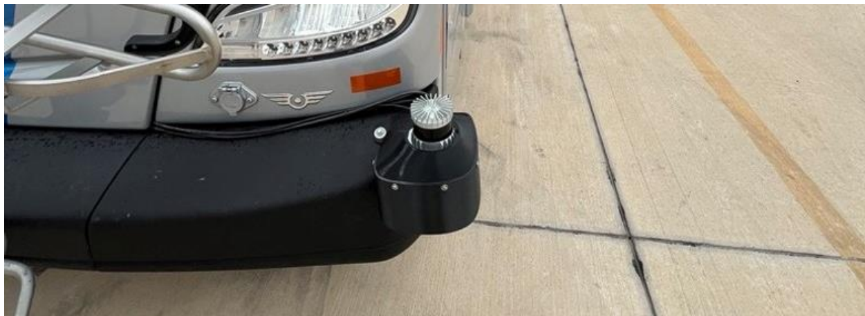
Figure 6-8: LIDAR and Radar (inside enclosure) mounted to the front bumper of CapMetro bus 8002
