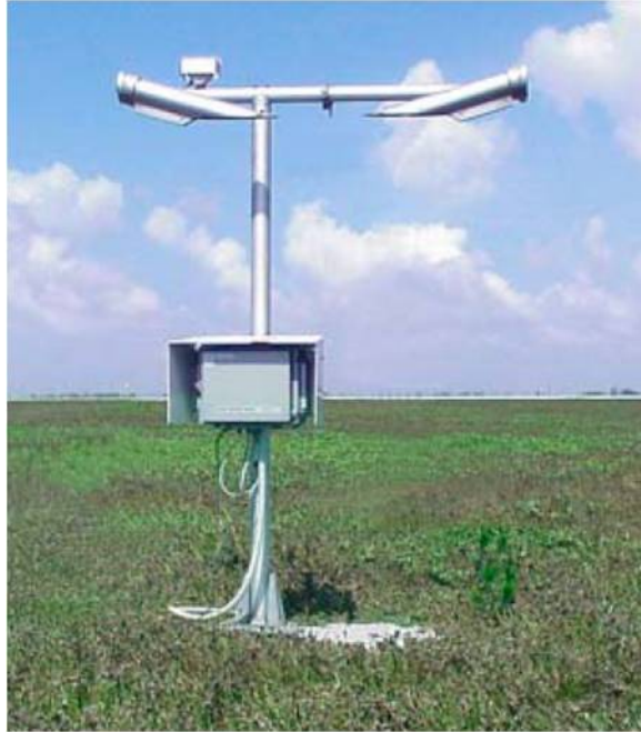
FIGURE 2-6 Vaisala Weather Sensor FD12P (22)
