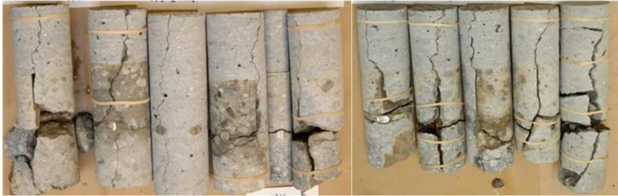
Figure 8. Cores from the Distressed Area of the Bonded Overlay Section
