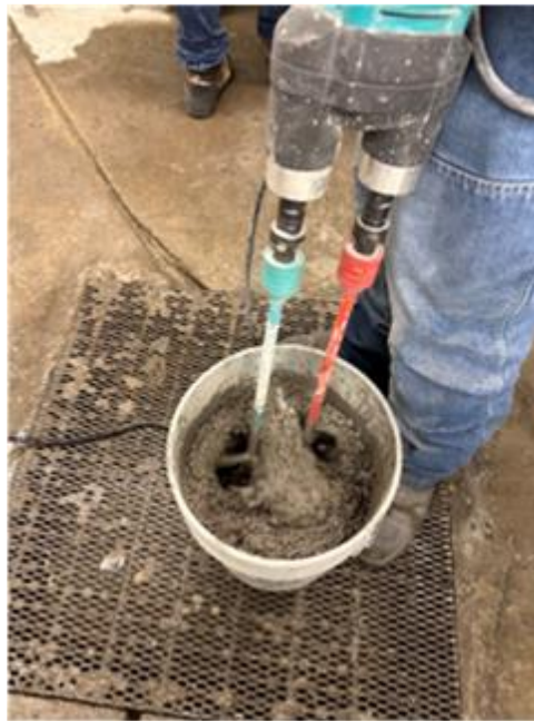
Figure 7. Mixing Engineered Cementitious Composite with Dual Paddle Mixer for Small-Scale Durability Samples
