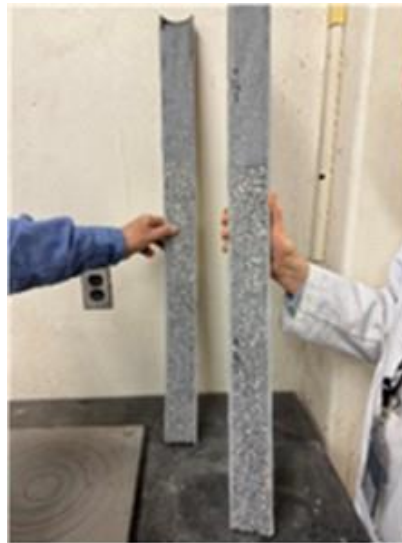
Figure 12. Mixture with Extra Water and High Slump Flow of 30 Inches Exhibited Segregation
