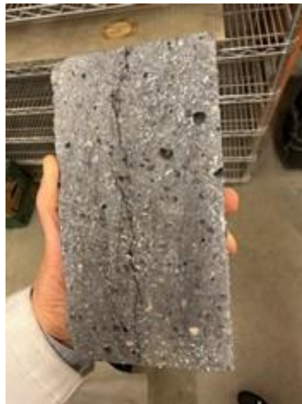
Figure 20. Well-Distributed Steel Fibers in Very High-Performance Concrete Used in Bristow Road Bridge Repairs
