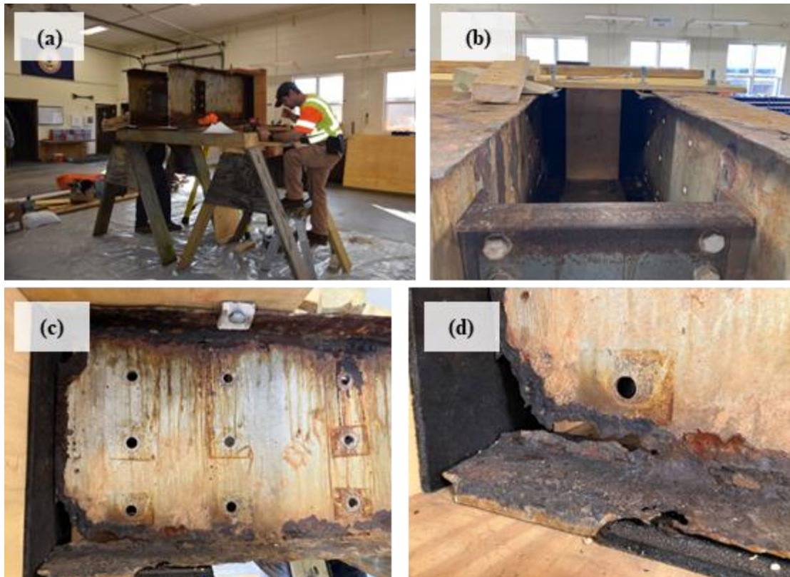
Figure 5. Photos of the Mockup Test Setup: (a) Overall View of Two Retired Bridge Beams; (b) Closeup View Between Beams; (c) Side View of One Beam; (d) Closeup of Corrosion Damage to One Beam
