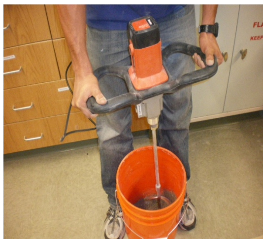
Figure 3.3 : Soil Mixing in Bucket Using Mechanical Mixer
