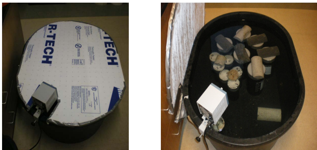
Figure 4.3: Stabilized Subgrade Soil in the Curing Tank
