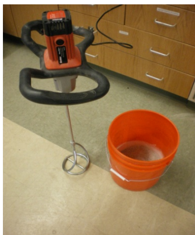
Figure 3.3 : Soil Mixing in Bucket Using Mechanical Mixer
