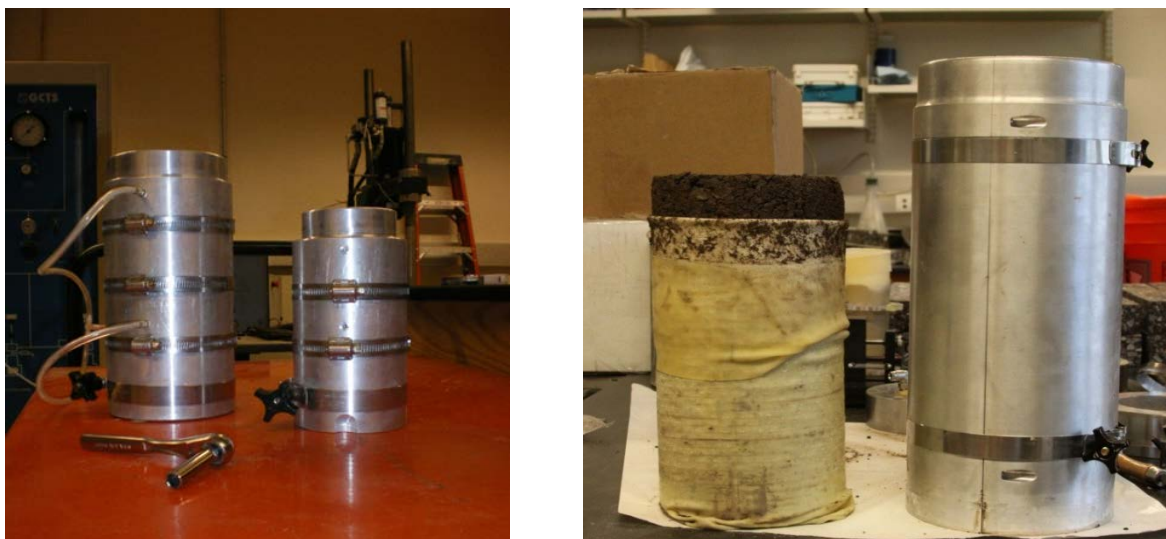
2.8" and 4" diameter subgrade soil mold 6" diameter base soil mold with compacted soil
