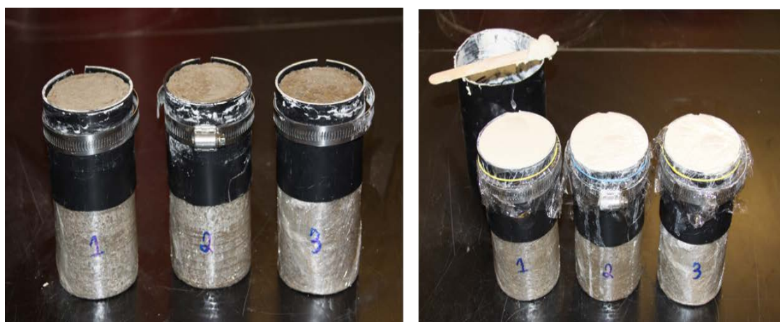
Figure 4.4: Capped Plastic Wrap Subgrade Samples
