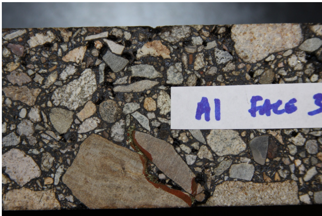
FIGURE 52 Fatigue Cracking in HMA Beam Sample SP-II-A1
