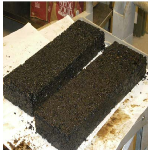
FIGURE 13 HMA Beam Samples Compacted by Linear Kneading Compactor
