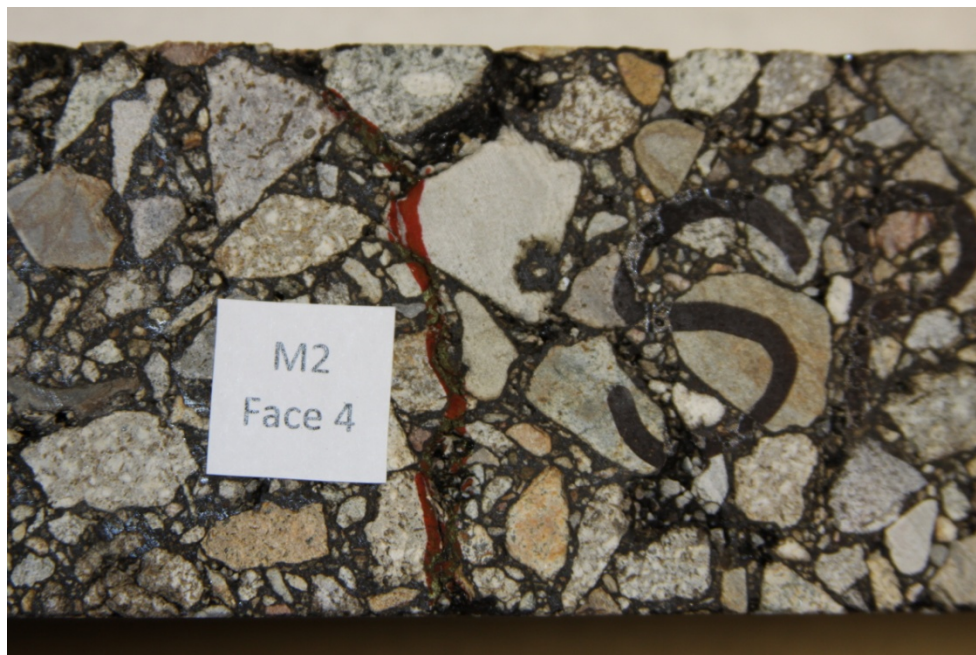
FIGURE 59 Fatigue Cracking in HMA Beam Sample SP-III-M2
