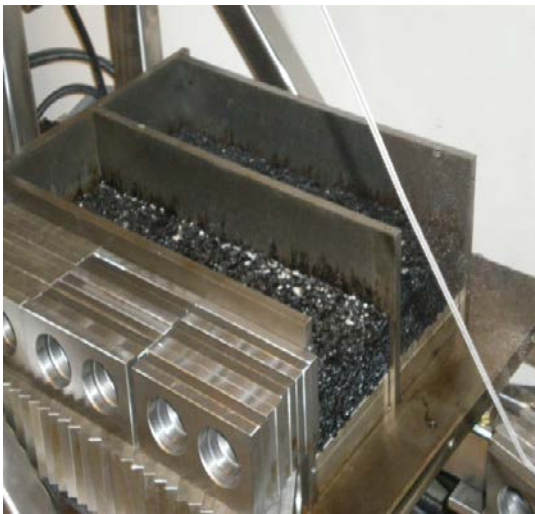
FIGURE 13 HMA Beam Samples Compacted by Linear Kneading Compactor
