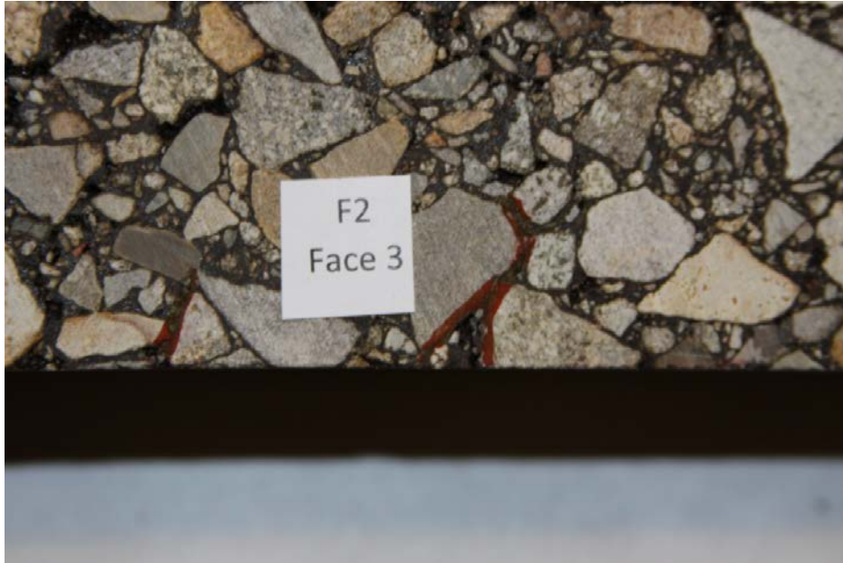
FIGURE 57 Fatigue Crack Propagating Upwards in HMA Beam Sample SP-III-F2
