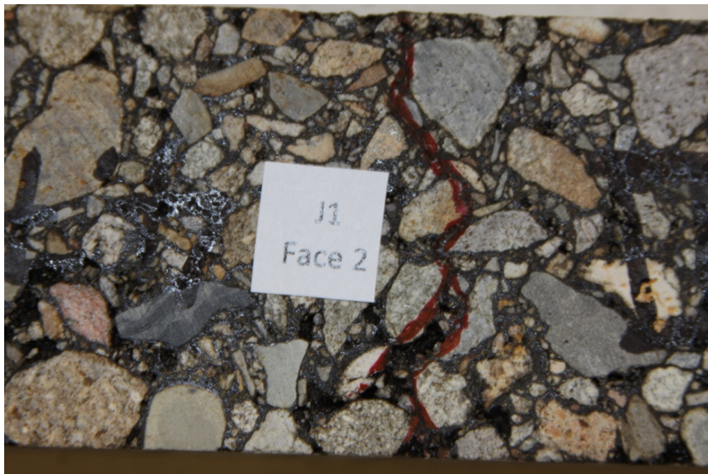
FIGURE 57 Fatigue Crack Propagating Upwards in HMA Beam Sample SP-III-F2
