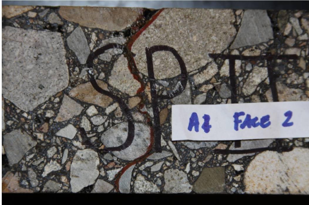
FIGURE 52 Fatigue Cracking in HMA Beam Sample SP-II-A1
