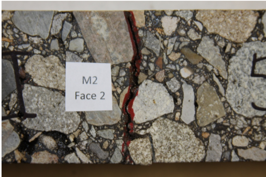
FIGURE 54 Fatigue Cracking in HMA Beam Sample SP-II-M2
