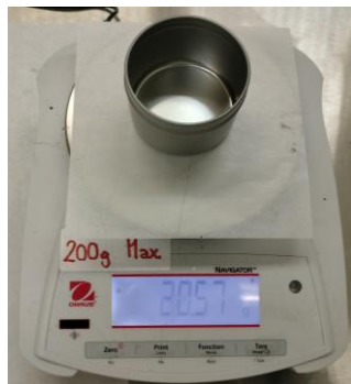
Figure 4.17. Empty can for cutback residue recovery being weighed on scale.
