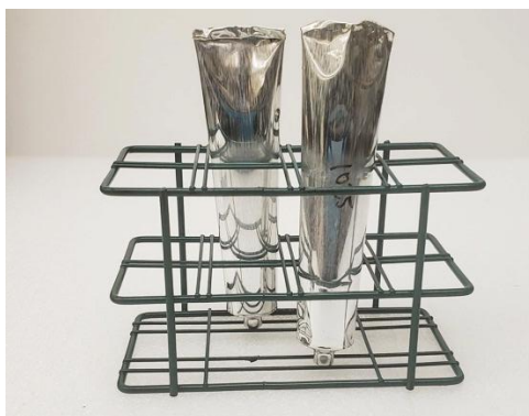
Figure 4.3. Cigar tube with sample; top of the tube is folded and crimped by hand to seal the sample.
