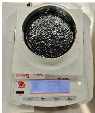
Figure 4.28. Emulsion residue being weighed after the specified time in vacuum oven.
