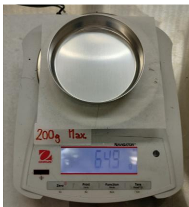
Figure 4.24. Empty container for emulsion residue recovery being weighed on scale.
