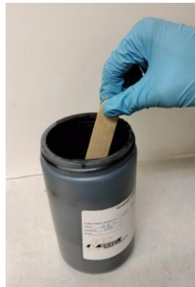
Figure 4.23. Emulsion sample being stirred thoroughly.
