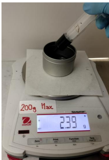
Figure 4.18. Required amount of cutback sample being poured in the can.
