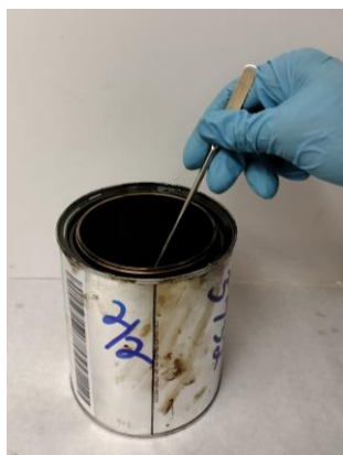
Figure 4.16. Cutback sample being stirred thoroughly.
