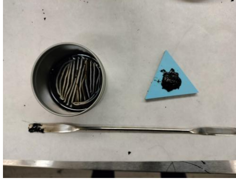
Figure 4.22. Scraping the cutback residue for testing in DSR.
