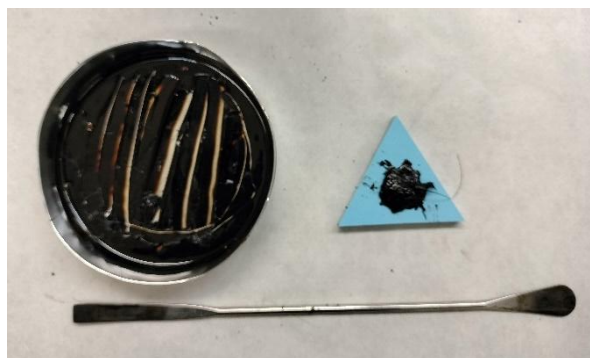
Figure 4.29. Scraping the emulsion residue for testing in DSR.
