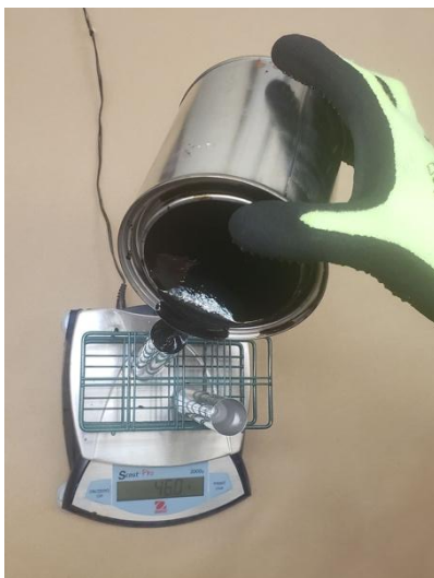
Figure 4.2. Sample being poured into the cigar tube.
