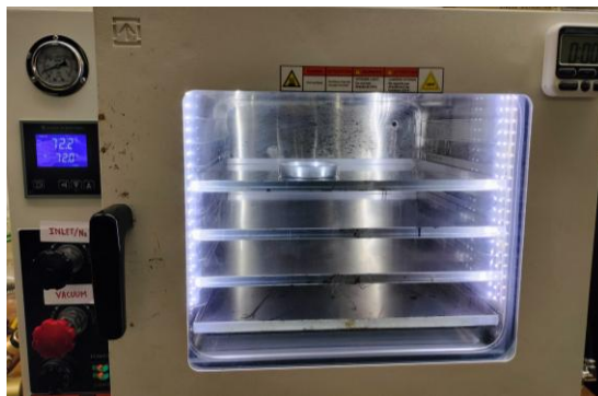
Figure 4.27. Emulsion sample in vacuum oven under the required pressure for residue recovery.
