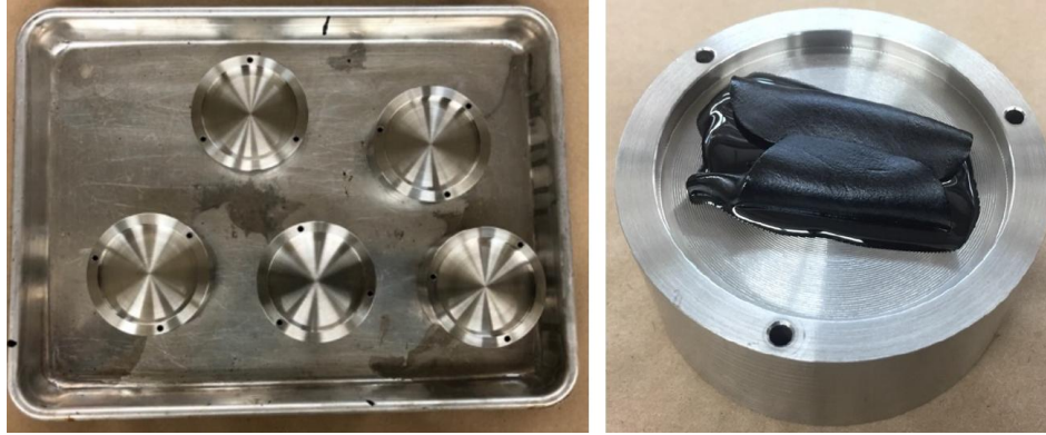
Figure 4.67. Bottom plates for five poker-chip samples (left) and one bottom plate with a binder sample placed in it (right).
