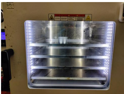
Figure 4.20. Cutback sample in vacuum oven 4 under the required pressure for residue recovery.
