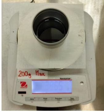
Figure 4.21. Cutback residue being weighed after the specified time in vacuum oven.
