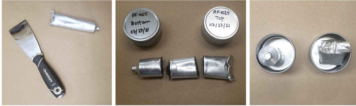
Figure 4.4. Cigar tube is cut into three after removing from the freezer (left: before cutting, middle: after being cut into three parts, right: top and bottom parts placed in cans).
