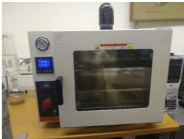
Figure 1. An example vacuum oven
