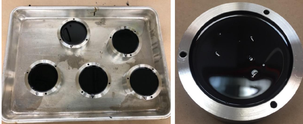
Figure 4.68. Bottom plates for five poker-chip sample discs with binder samples (left) and one bottom plate with the three spacer dowels dropped on top of the binder surface (right).
