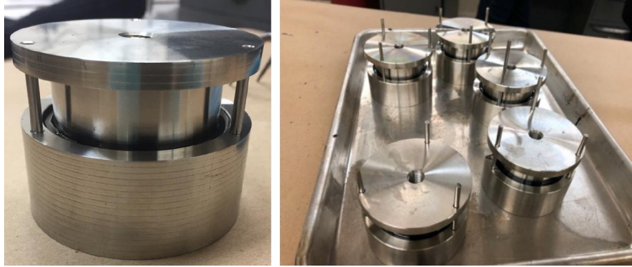
Figure 4.69. A poker-chip sample that sandwiches the binder specimen between the top and bottom pieces that are aligned using three pins (left); five complete discs ready for temperature conditioning and testing (right).
