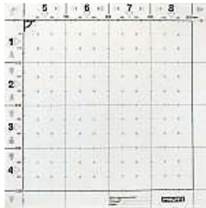
Figure 5.1. 2 ft. x 2 ft. reference grid used for Hilti PS 250 Ferroskan.
