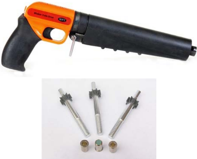
Figure A.6 Driver and probes of Windsor Probe System WP-534 (Windsor 2010).
