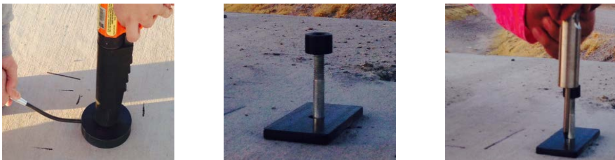
Figure A.8 Windsor probe penetration test
