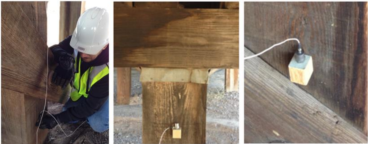
FIGURE 26 Accelerometers Mounted on a Pile by Wooden Blocks.
