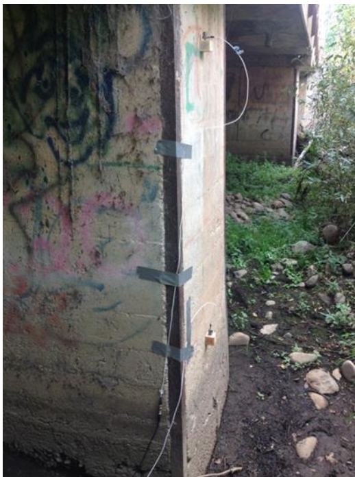
FIGURE 134 Attached Accelerometers on the Pier Side
