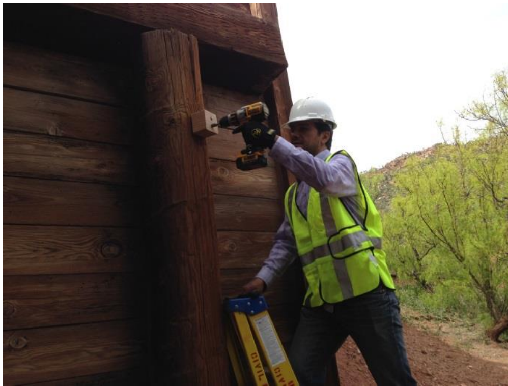
FIGURE 25 Attachment of a Wooden Striking Block onto the Test Pile
