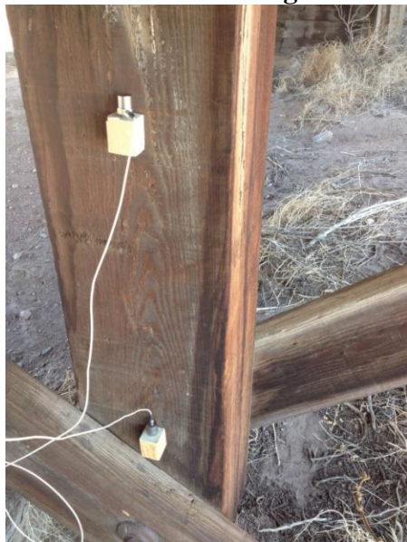
FIGURE 118 Accelerometers Attached onto a Pile
