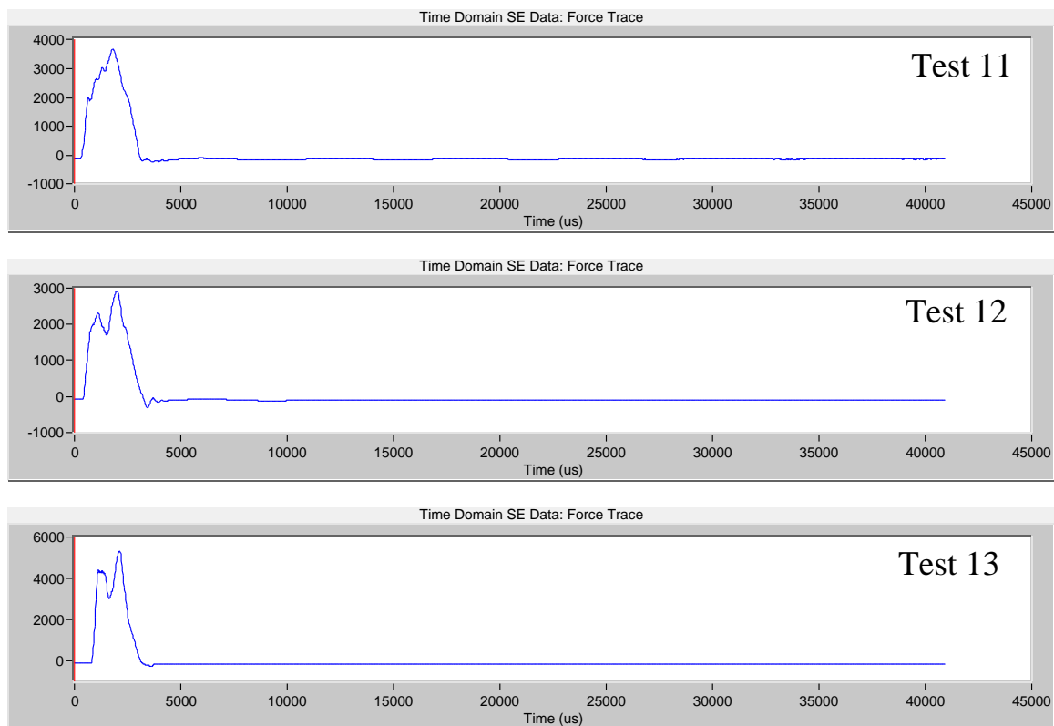
FIGURE 78 Initial Impulse from the Hammer's Force Sensor (Wooden block, Hard-tip)
