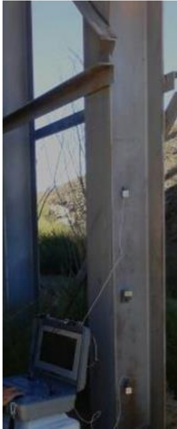
FIGURE 128 SE Test Setup for a H-pile of Bridge No. 7480
