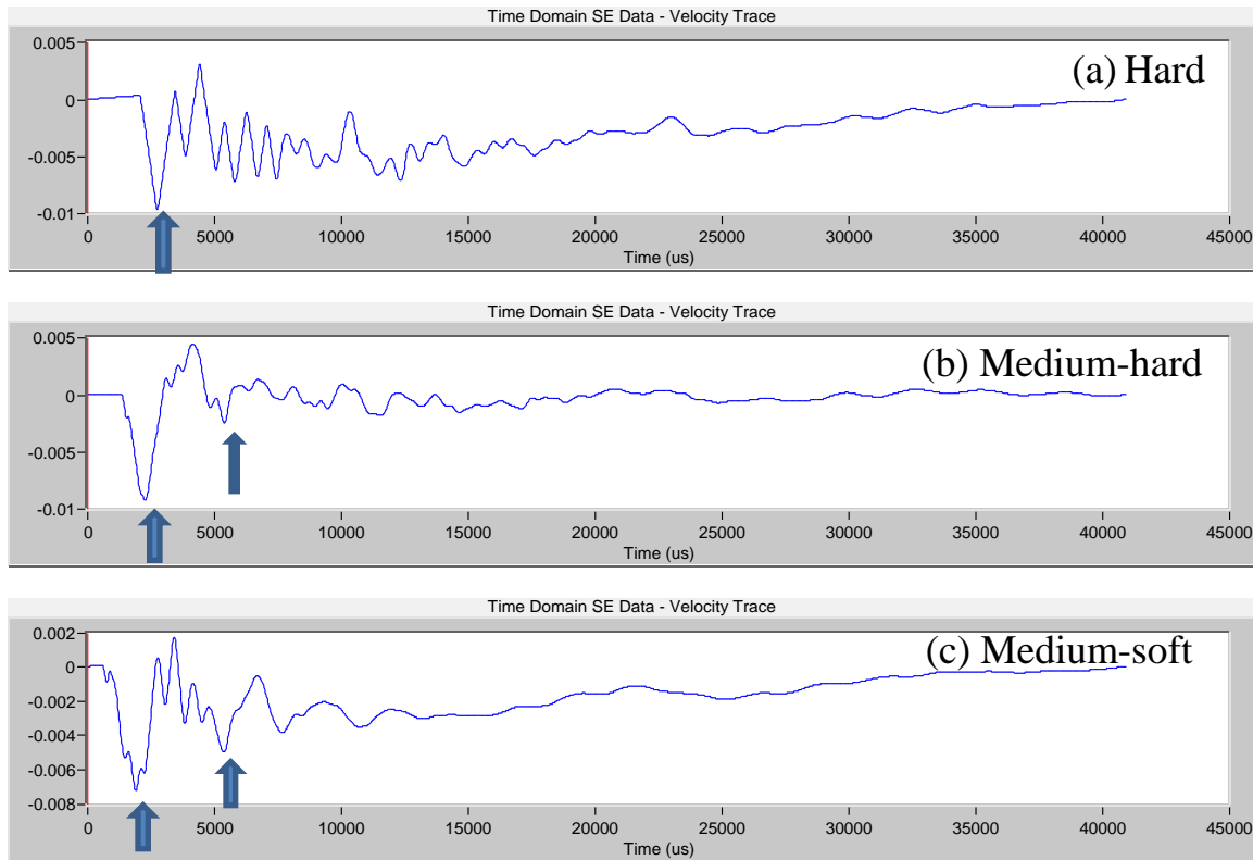
FIGURE 98 Velocity Graphs Obtained by Striking with Different Hammer Tips (Pile B)
