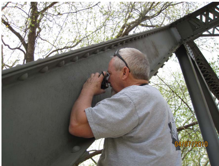
Figure 2.8 Measuring Coating Thickness with a Tooke (Scratch) Gage
