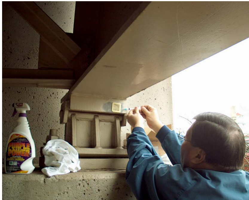
Figure 2.10 Bresle (Patch) Test to Measure Soluble Salt Contamination
