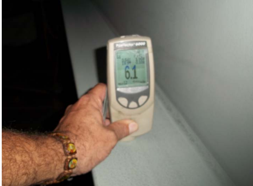
Figure 4.15 Dry Film Gage
