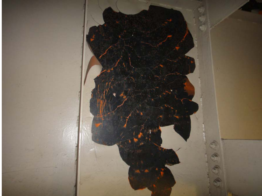
Figure 1.5 Aged Lead-Alkyd Sheeting-Type Complete Disbonding Failure from a Mill Scale Substrate
