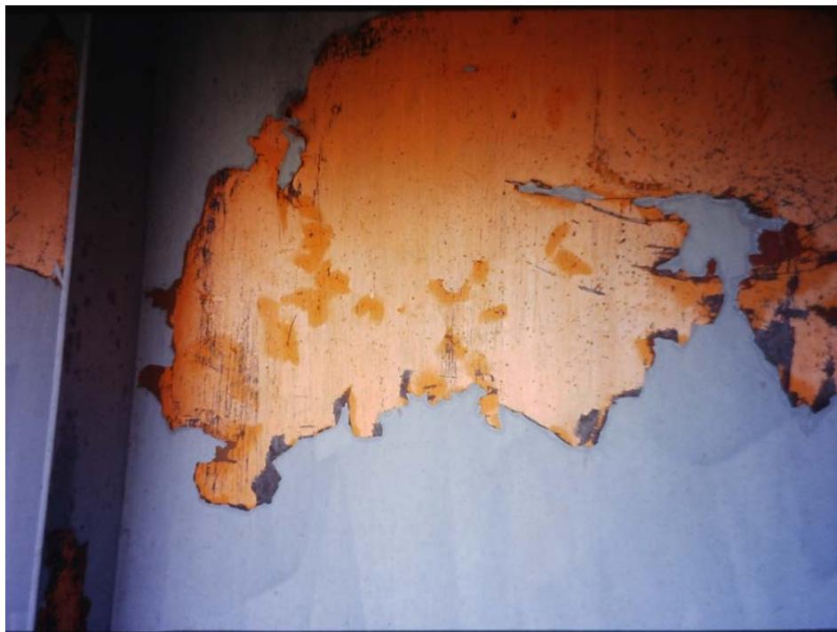
Figure 1.4 Intermediate Coat Adhesion Failure Between Lead-Alkyd Primer and Alkyd Topcoat
