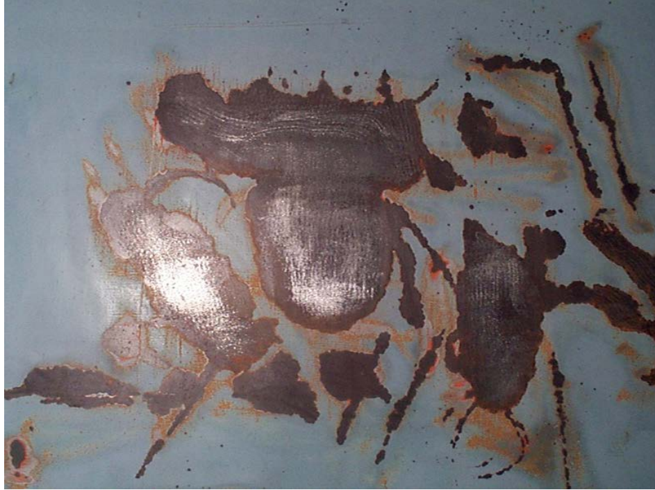
Figure 3.7 Surface Prepared to the SSPC SP-11 Standard. Note the typical abraded surface resulting from mechanical surface preparation.
