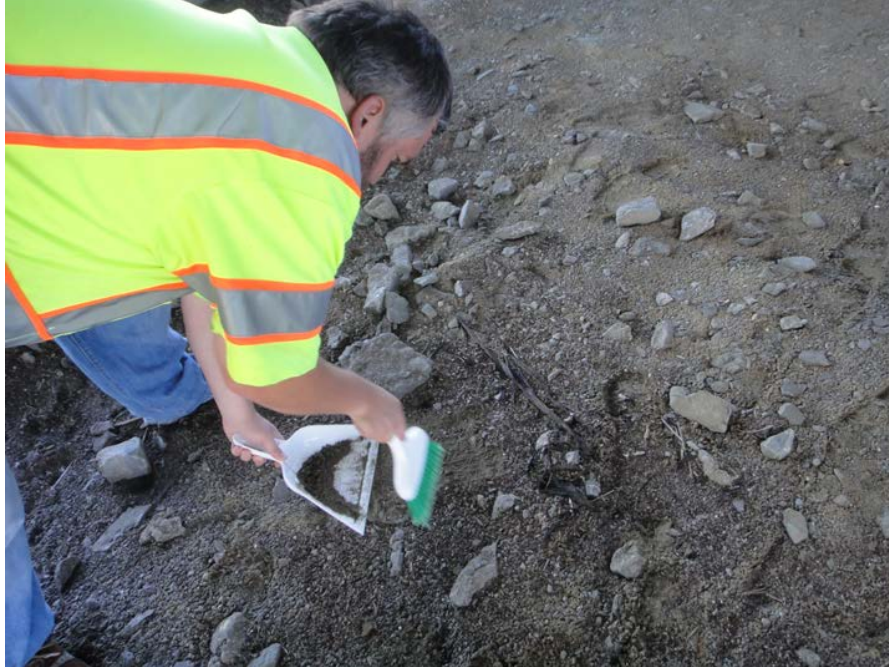
Figure 4.17 Worker Collecting a Soil Sample on Project that Involved Lead Paint Removal
