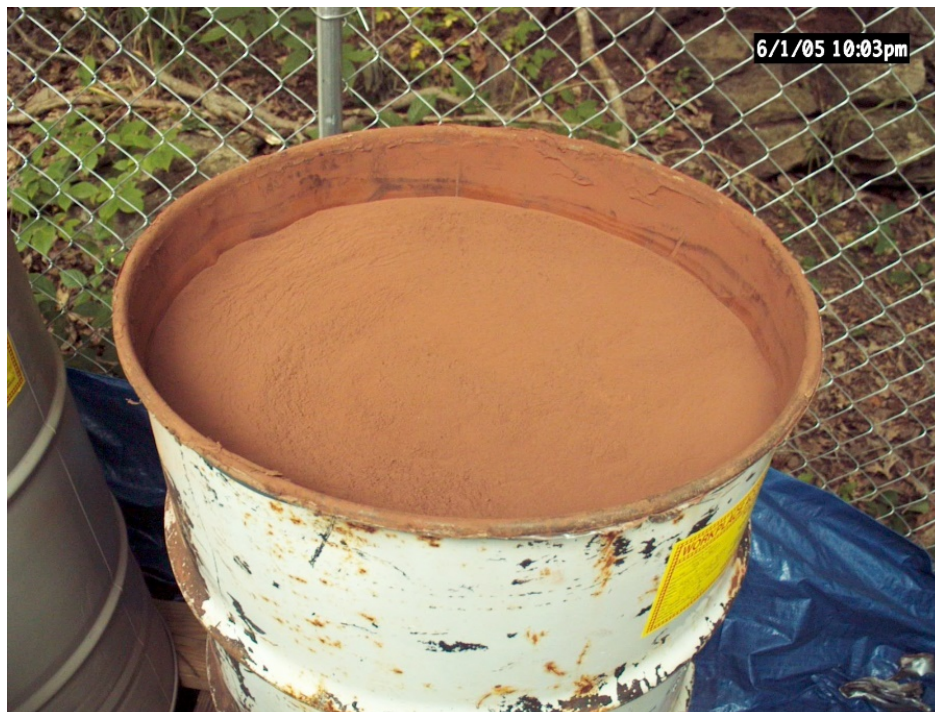
Figure 3.18 Lead-Contaminated Paint Debris
