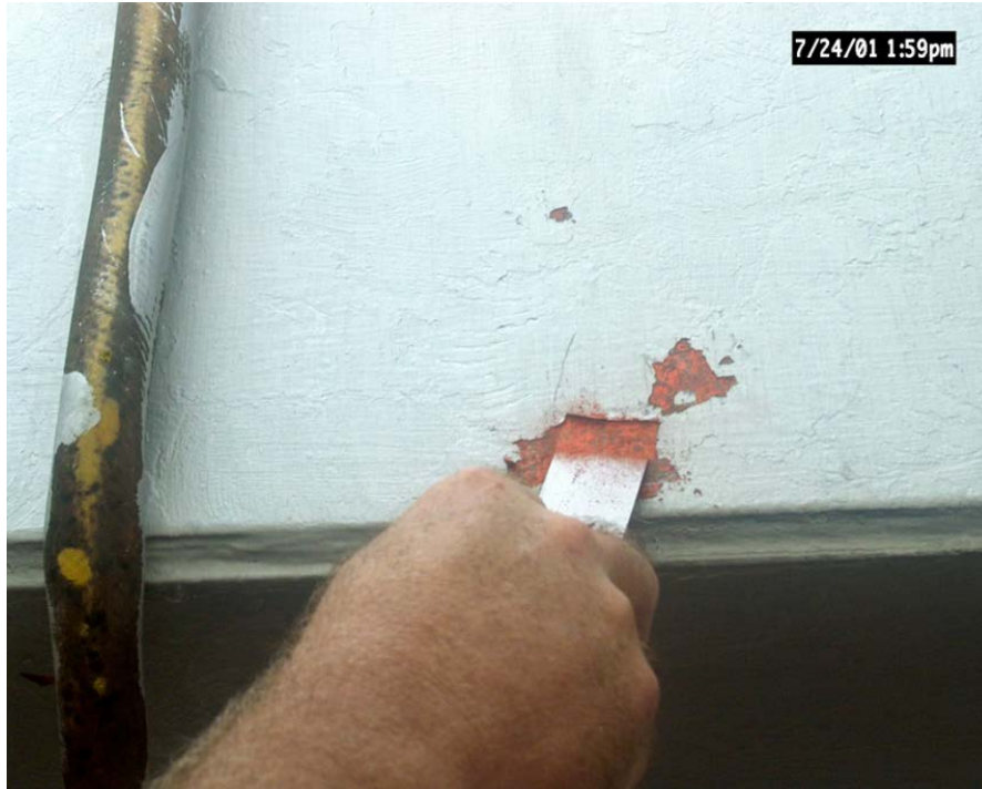
Figure 3.9 Probe of Coating Failure to Verify Adherence.
