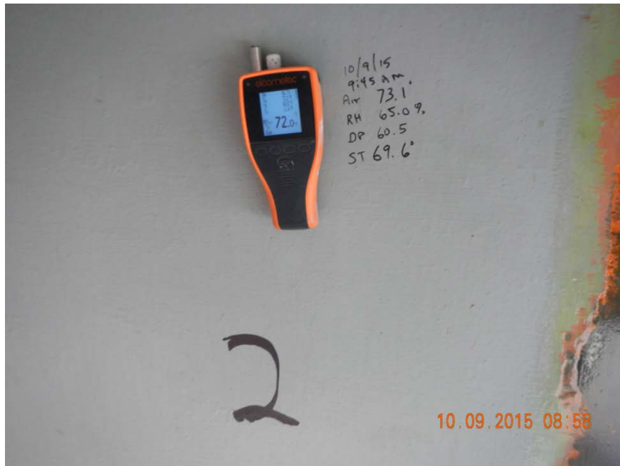
Figure 4.9 Electronic Dew Point Gage
