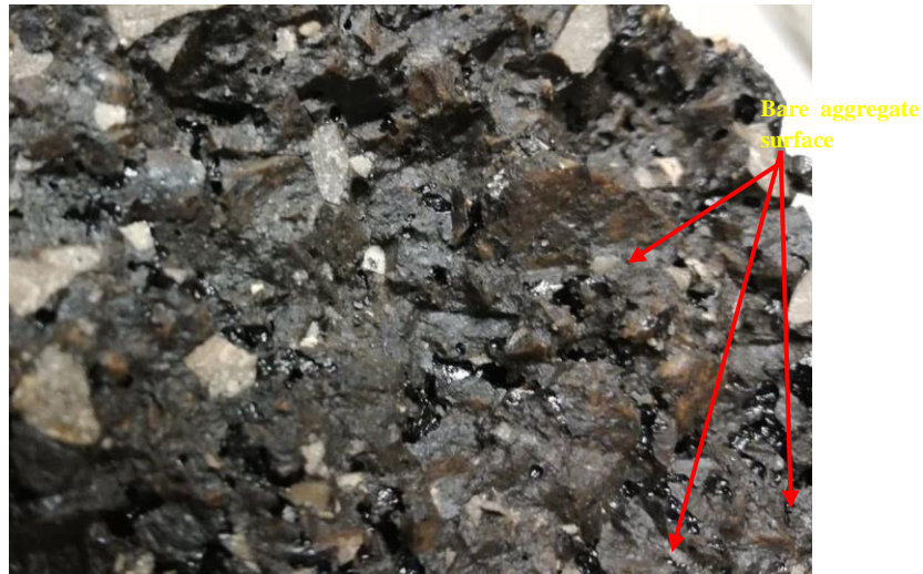
(c) Fracture face after DCT test
