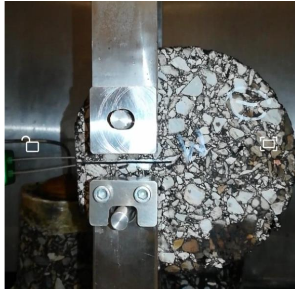
(b) DCT test in progress
