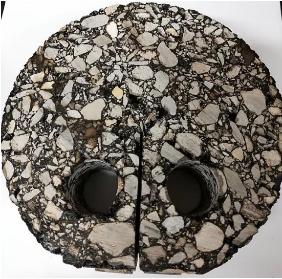
(a) A prepared sample for DCT test
