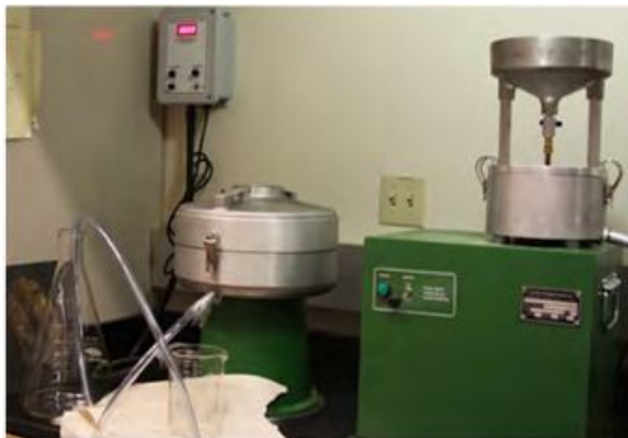
(c) Fines separation through centrifuge
