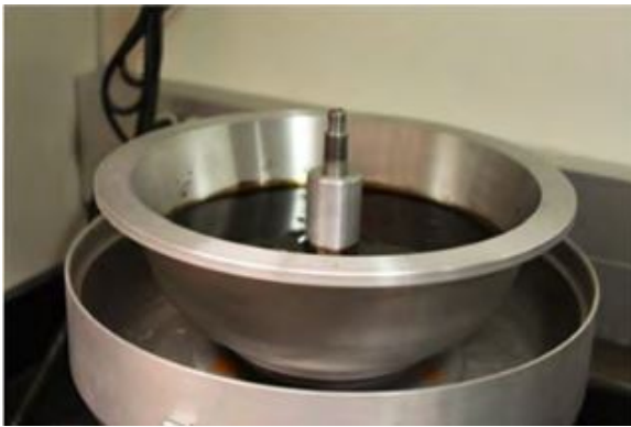
(a) Asphalt mix in Trichloroethylene
