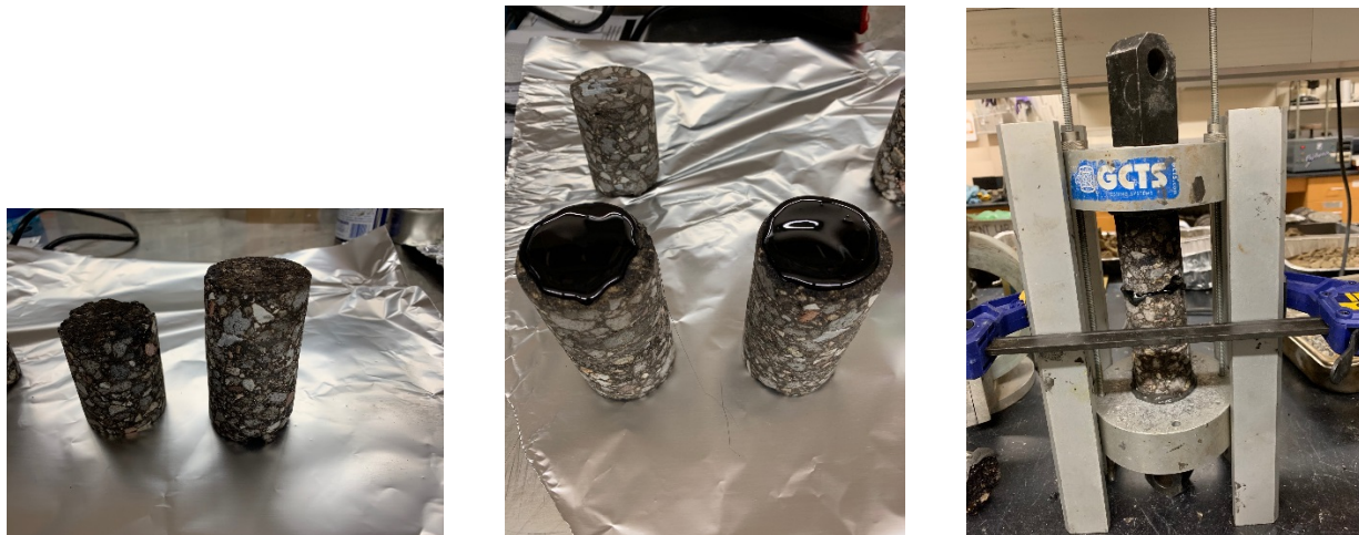
FIGURE 106 Sample preparation for the TSRST test
