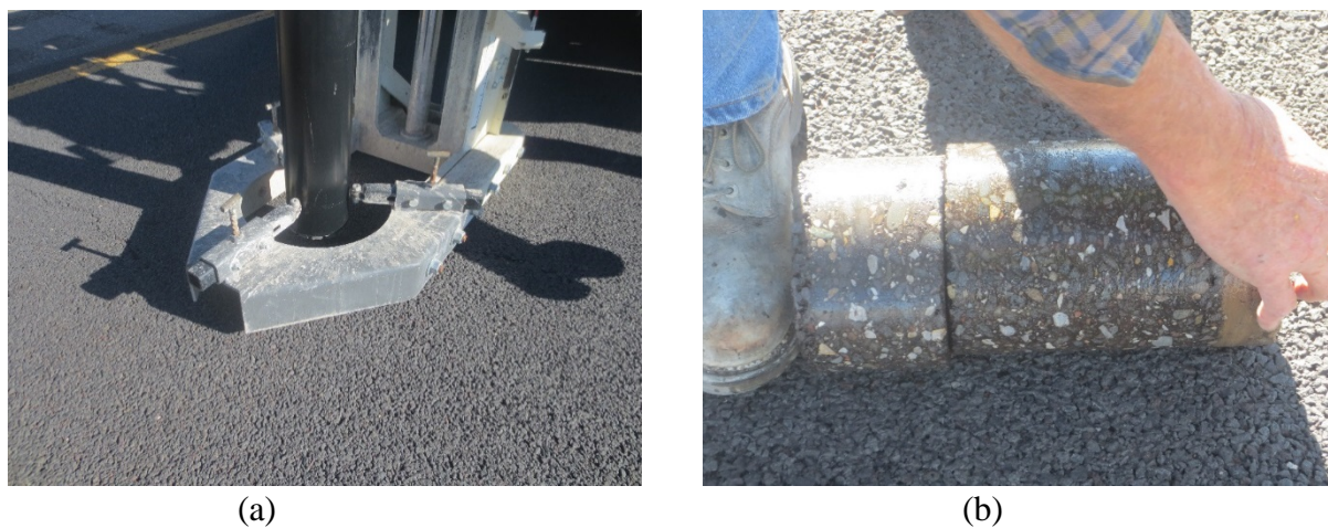
FIGURE 45 AC core from passing lane
