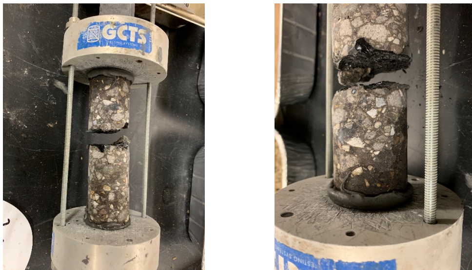
FIGURE 107 Delamination in the TSRST test
