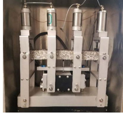
(b) Beam sample in test setup
