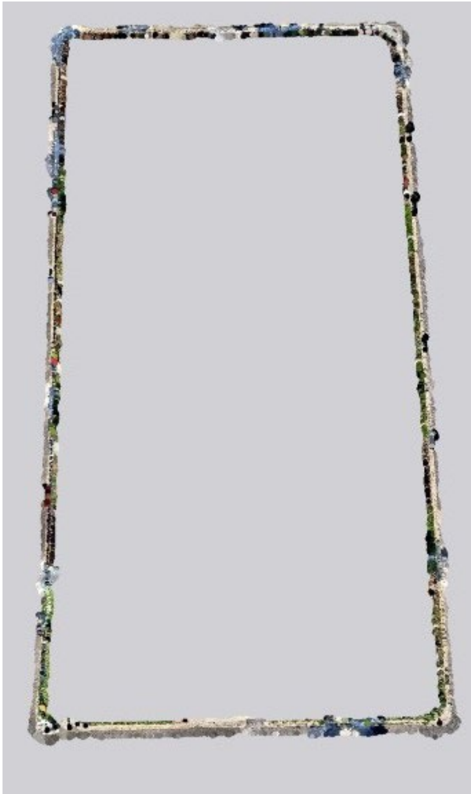
Figure 6.7 iPhone Point Cloud Dataset Whole City Block from 3D Scanner LiDAR Application
