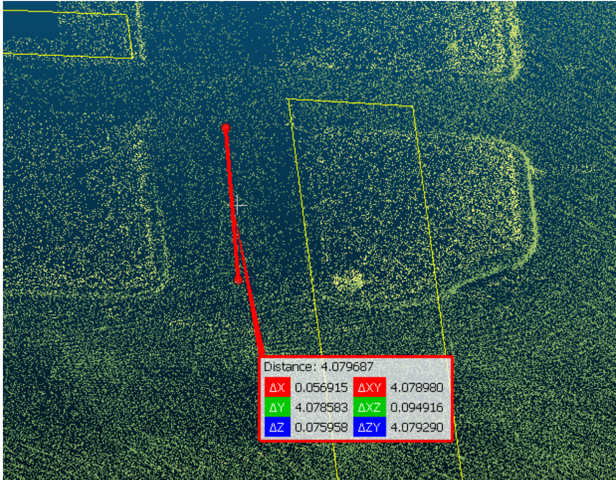
Figure 11.8 Curb Ramp Running Slope Measurement in Cloud Compare
