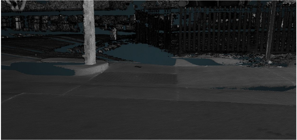
Figure 4.14 Trimble TX8 Point Cloud Dataset 28th Avenue and Eudora Street South Curb Ramp
