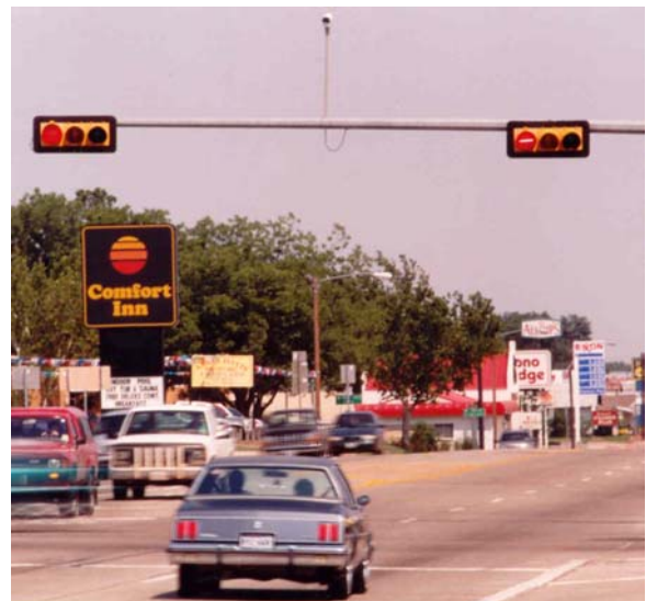
Figure 6-14. Strobe-Enhanced Signal Heads.
