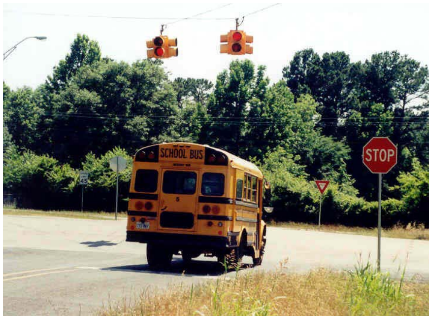
Figure 6-10. Intersection Flashing Beacons.
