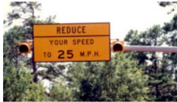
Figure 7-24. Flashers Activated When Speeds Exceed 30 MPH.
