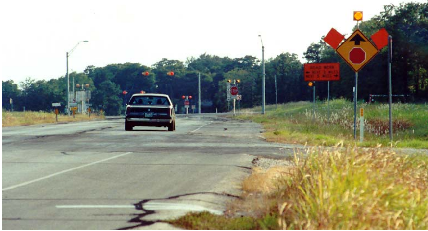
Figure 7-42. Orange Warning Flags on Stop Ahead Sign.
