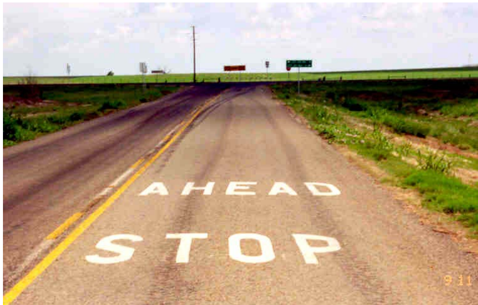
Figure 6-2. Example of Advance Warning Pavement Markings.
