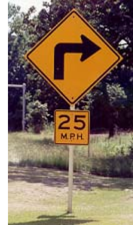
Figure 5-22. Example of Advance Sign for a Horizontal Curve.
