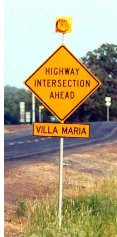
Figure 6-3. Example of Flasher on Advance Intersection Sign.
