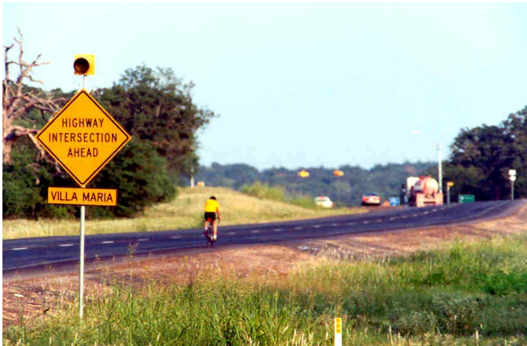
Figure 7-45. Solar-Powered Flashers on Intersection Warning Sign.
